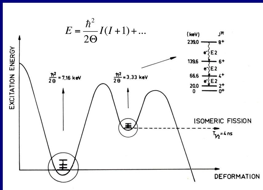
Fit of the E2 energies to the QM rotator
