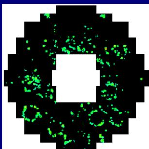
Low field (air coils), limited tracking → limited resolution
