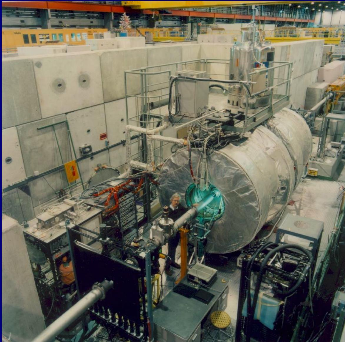
UV-photon detectors based on photo effect in TMAE vapor at 40°C
