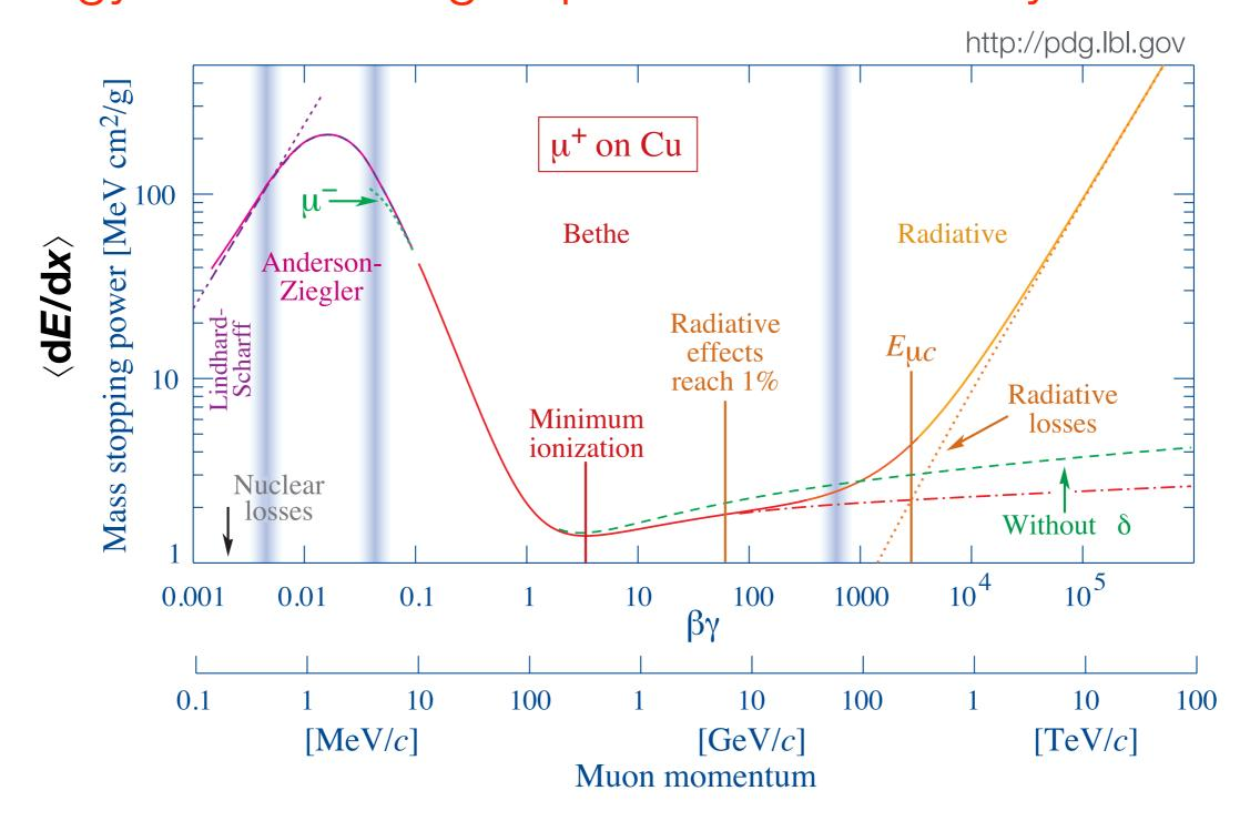
$\mu^+$  on Cu: Radiational energy loss ("bremsstrahlung") starts to dominate over collisional energy loss ("Bethe-Bloch") for  $p \gg 100~{\rm GeV}/c$
