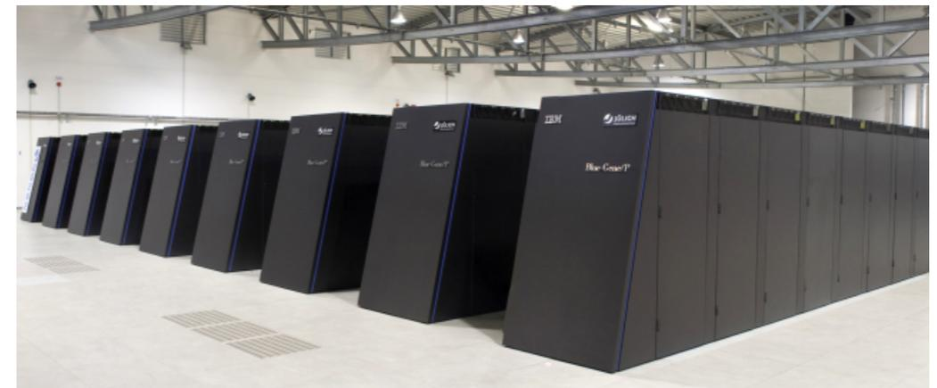
Example of a machine for lattice QCD: JUGENE in Jülich (294,912 processor cores,  $\sim 1$  PetaFLOPS)
