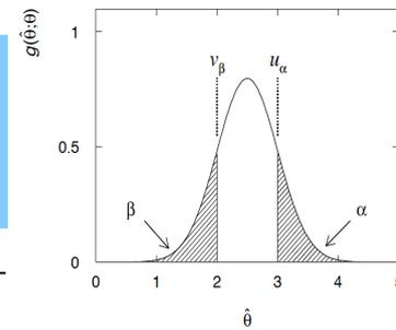
See how the functions  $u_\alpha(\theta)$  and  $v_\beta(\theta)$  can be as a function of the true value of  $\theta$
