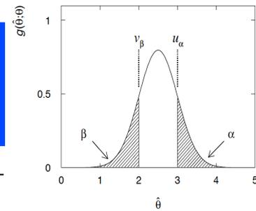
If the form of the estimator pdf  $g(\hat{\theta})$  is not Gaussian, then the 'standard deviation' definition of statistical error bars does not hold!
