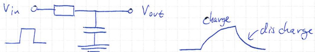
$$V_{in} = RC \frac{dV_{out}}{dt} + V_{out} \quad (\text{using } I = \frac{dQ}{dt} = C \frac{dV_{out}}{dt})$$
