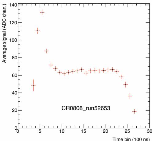
Figure 3: Average pulse height as a function of time
