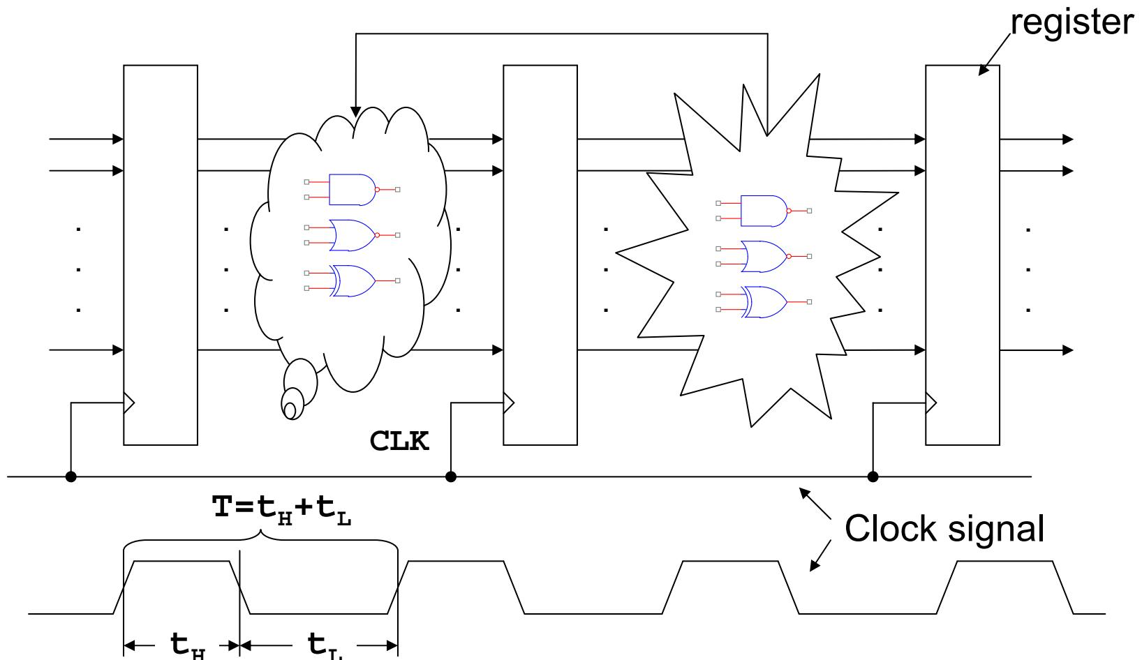
At each rising clock edge the registers memorize the current values at their inputs. The outputs are updated after some small delay  $t_{CO}$
