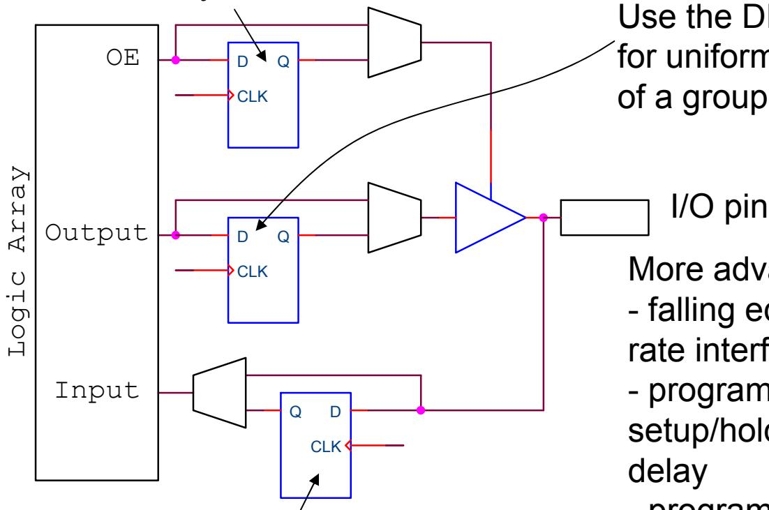
Use the DFF in the input path for uniform and predictable setup/hold times of several I/Os, e.g. a data bus with 32 bits.
