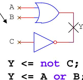
Example for pull-up (weak 1) and tri-stated outputs, **std\_logic** is required
