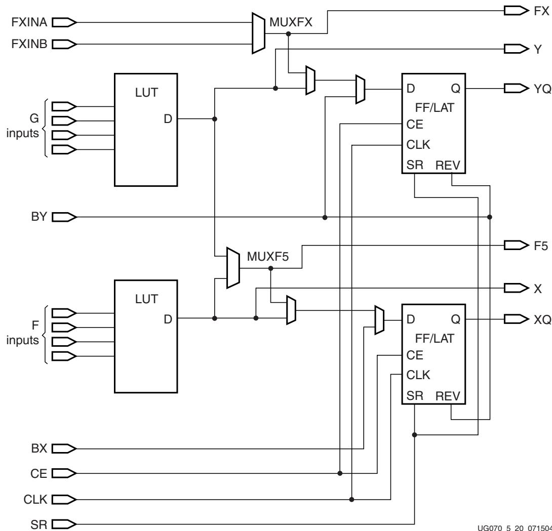
Each SLICE contains two LUT4, two FFs and MUXes. The two LUT4 can be combined into one LUT5.
