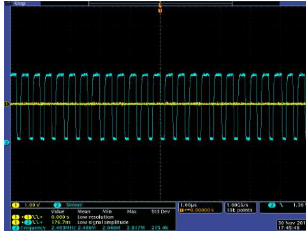
Figure 10.9: Comparator oscillation monitored with the oscilloscope at threshold 0.79V.
