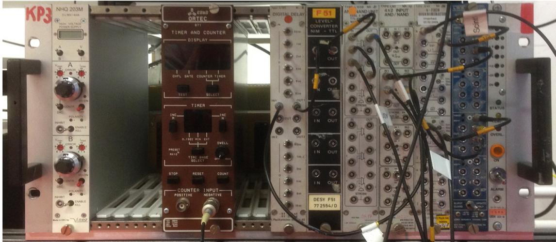
Figure 7.3: Picture of the trigger electronics. From left to right: High voltage power supply, scaler, delay unit, NIM to TTL converter, TTL NAND-logic, AND-logic, discriminator, discriminator.
