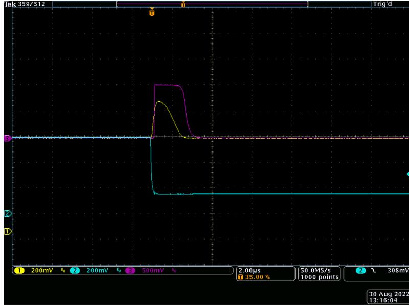
Figure 5.3: Test outputs of AP3.1 measured with an oscilloscope. Blue shows the injection pulse created by discharging the injection capacitor. Yellow: Amplified injection pulse. Magenta: Digital signal of the comparator caused by the injection pulse. The comparator pulse is shaped by the receiver unit in the periphery.
