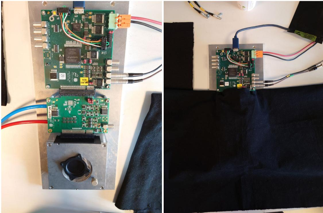
Figure 4.2: Setup with a cooling jig and with (right) and without (left) blanket for light protection during measurements. As the cooling jig is used for multiple purposes, it features a cutout for holding a radioactive source. Additionally, the biasing, powering connections, and cooling water tubes are shown.
