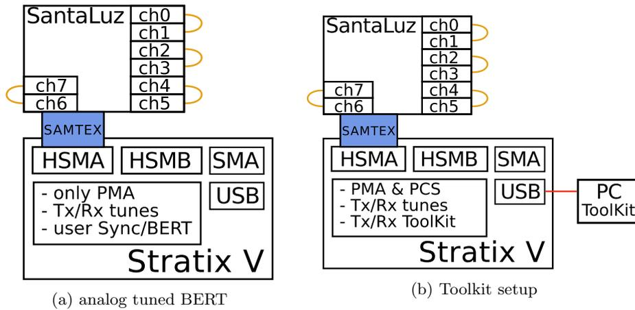
Figure 5.18: Setup for analog tuned transceivers.
