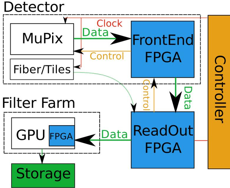
Figure 1.7: MuPix readout chain with data connections in green, control in orange, clock in red and all FPGAs used for the chain in blue.
