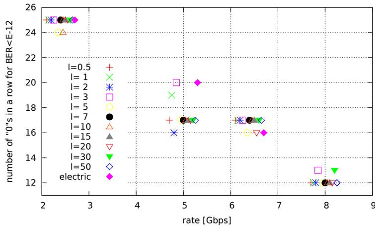
(b) Number of maximal zeros followed by a alternating zero-one pattern filling up 64bit words at a given rate. The data is shifted around the actual used rates of 2.4, 5, 6.4 and 8 Gbit/s to achieve a better visibility.
