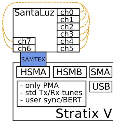
Figure 5.14: Setup scheme used to measure the performance of the different cages. Only one optical fiber is used at the time.
