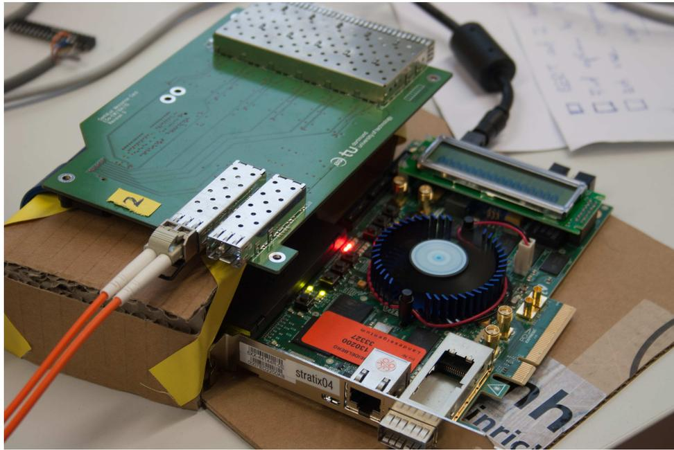
Figure 5.10: Setup to test optical SFP links. A SantaLuz mezzanine card (labeled with 2) is connected with blue Samtec high speed cables on HSMC port A of a Stratic V development board. The LCD display, a fan right above the FPGA, Ethernet and QSFP plugs are visible. The mezzanine board is equipped with one optical SFP transceiver which is connected with a duplex multi-mode optical fiber in orange.
