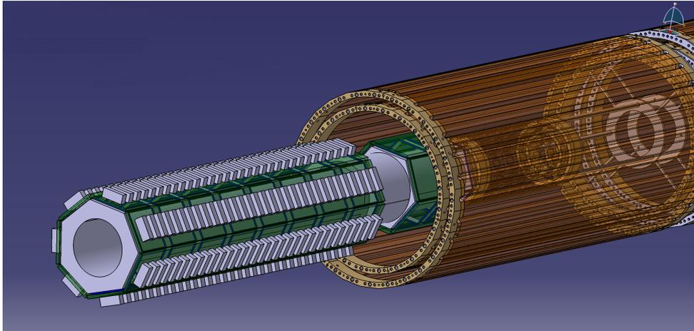
Figure 1.6: Mu3e phase 1 detector rendering with 4 layers of pixel detector, beam pipe and electronics in green. The available space for readout electronic is highly limited.
