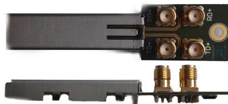
Figure 5.4: Top and side view of an electrical SFP plug.
