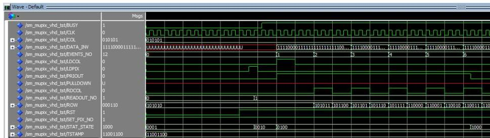
Figure A.4: An example view of ModelSim where a MuPix emulator RTL simulated is performed.
