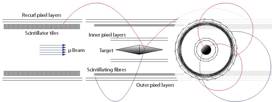
(b) Phase 1b: Added scintillating fibers and tiles, one recurl station on each side.
