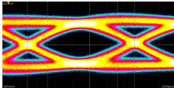
(c) well tuned eye:  $V_{od} = 26$ ,  $1^{st}_{post} = 11$ ,  $2^{nd}_{post} = 1$ ,  $pre = -2$
