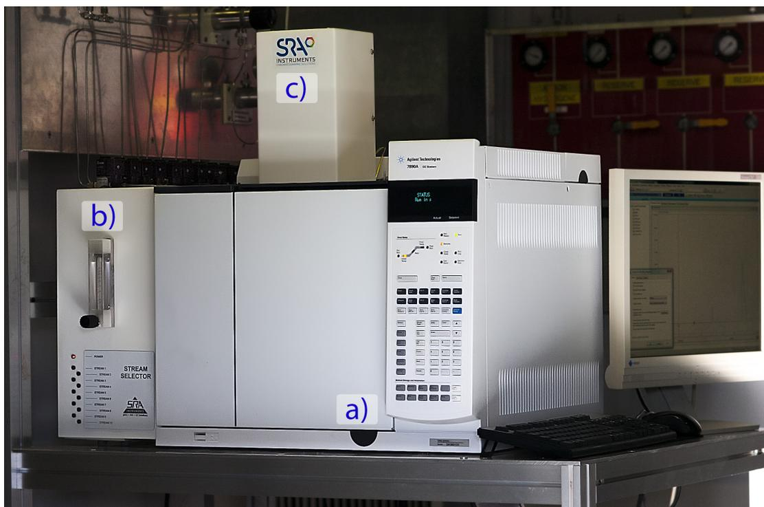
Figure 2.1.: The Agilent 7890A gas chromatograph (a) with the stream selector (b) and switching valves (c) by SRA.
