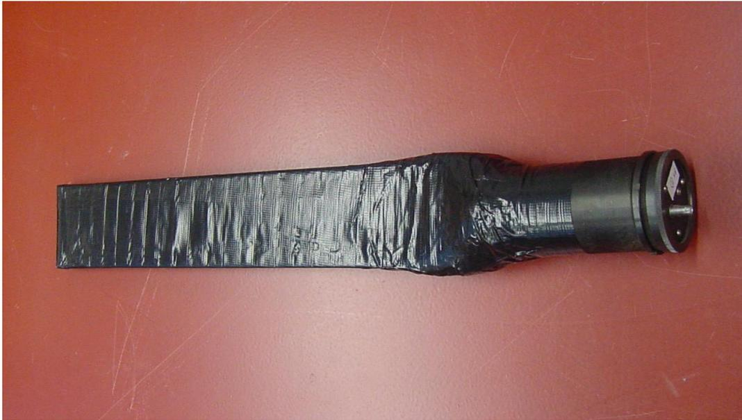
Figure 6.7: The whole scintillator assembly as it is used in the experiment. From left to right: scintillator pad beneath black tape; light guide beneath black tape; photomultiplier beneath mumetal<sup>®</sup> shielding; high voltage connector and signal output connector. The whole scintillator assembly is 870 mm long
