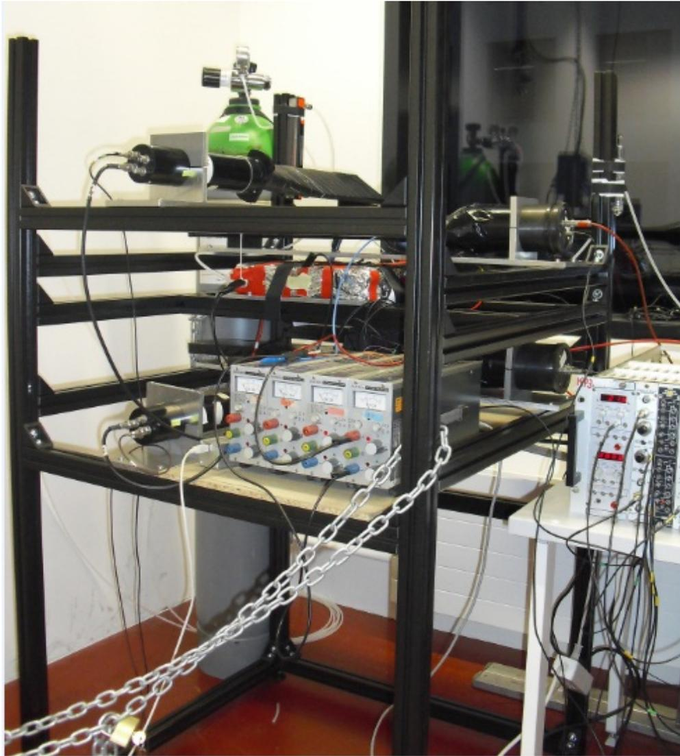
Figure 7.7: Picture of the mechanical installation supporting the individual components. The main support structure (black) holds the support structures of the individual components (silver, aluminium), the four scintillators (black) and the TRD chamber (wrapped in aluminium foil)
