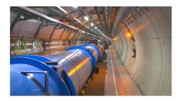
Figure 3.2.: Picture of the LHC with its superconducting magnets placed in the tunnel of the former LEP collider. Figure taken from Ref. [58]
