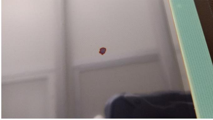
Figure 5.11: A dark, burnt spot that developed on a GEM during the recording of discharges in Ar-CO<sub>2</sub> (70-30). The area started to discharge rapidly at a potential difference across the GEM that was lower by about 30 V than usual. By using the method presented in Sec. 5.2.4, the GEM could be recovered. Afterwards, no (frequent) discharges occurred around the burnt area.
