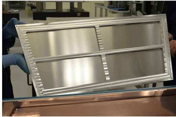
**Figure 17:** (i) the metal pins maintain the alignment of GEM and frame, (j) the gluing jig's cover plate
