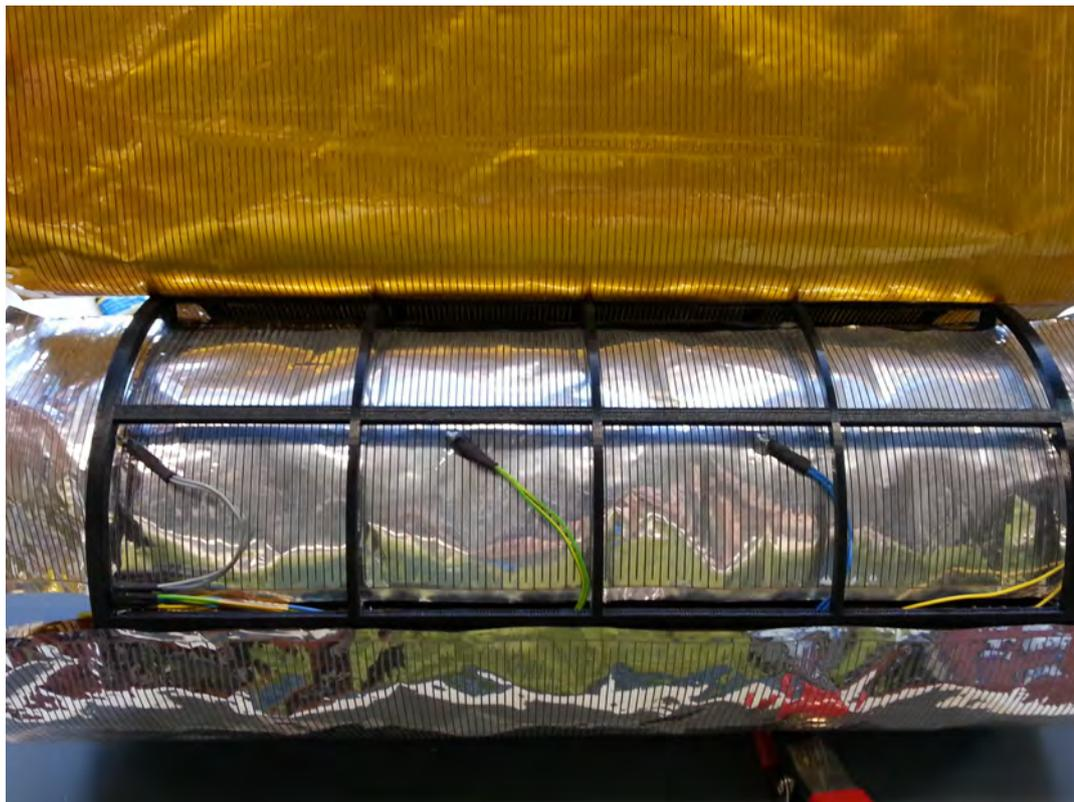
Figure 3.9: Four temperature sensors positioned on one of the inner foils. The glueing process is nearly completed.
