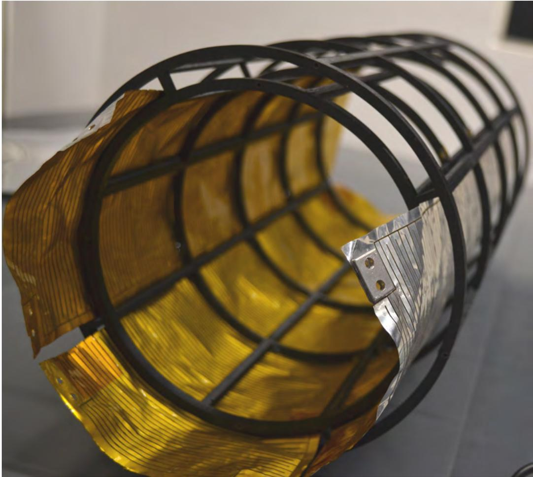
Figure 3.7: Foil supporting framework with three foils glued on.
