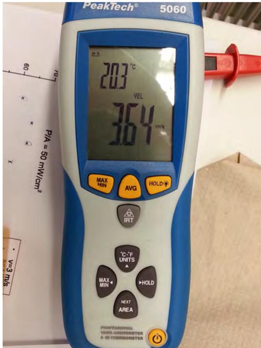
(a) The display of the anemometer with airspeed and temperature values.
