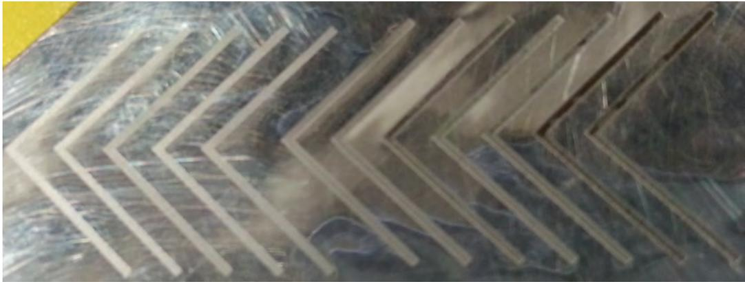
Figure 3.4: Tuning-pattern to adjust working parameters of the laser system
