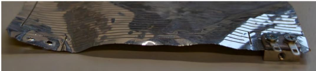
Figure 3.6: On the right: Connector mounted to a heating foil.
