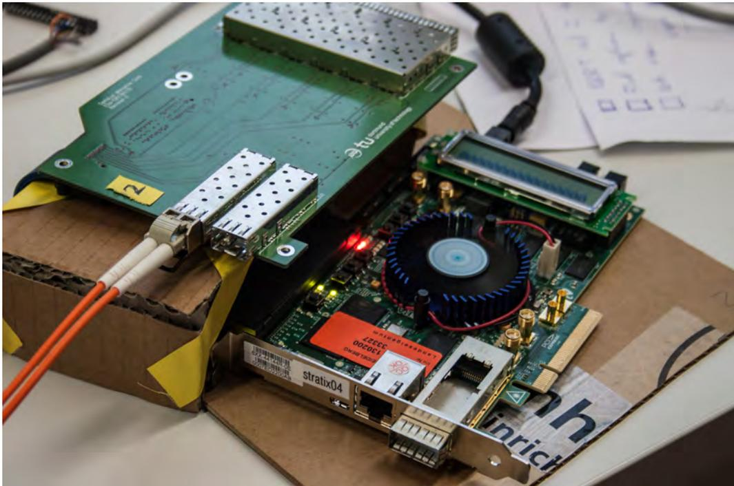
Figure 5.1: Picture showing the setup containing FPGA board, SantaLuz board, and SFP transceiver with optical fiber.
