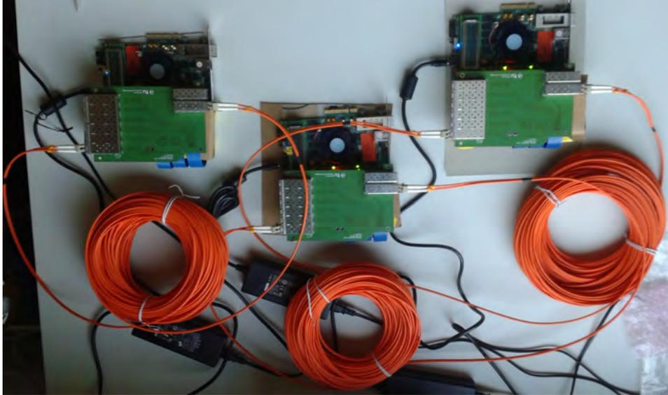
Figure 7.4: Setup for long term BERT at 6.4 Gbit/s using three FPGAs. The picture shows the setup for  $l=50$  m.
