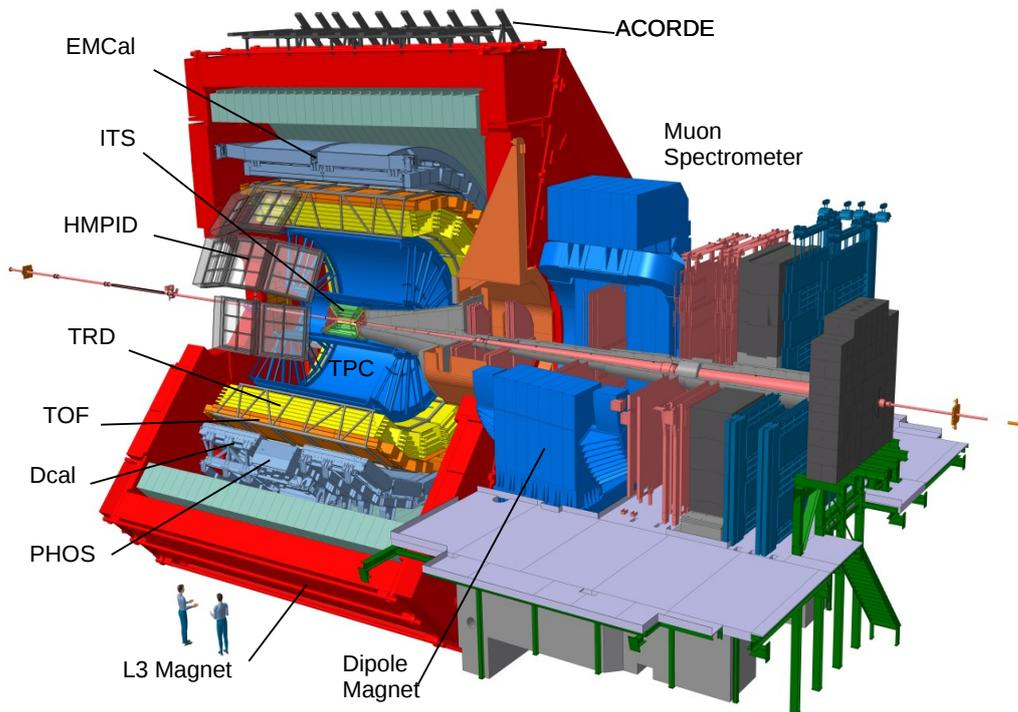
Figure 1.1: *Schematic view of the ALICE experiment at CERN and its main detectors [1].*
