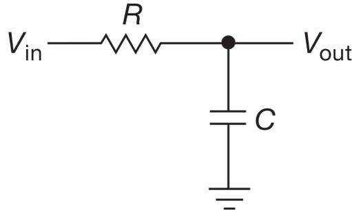
Figure 4.1: *RC low-pass filter [15].*
