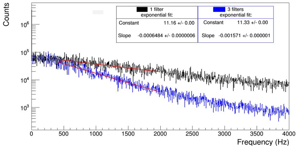
Figure 4.4: Frequency spectrum of white noise signal when applying one (black) and three (blue) filters. Data fitted with the exponential function. The slope values are indicating that the roll-off is increasing when applying more filters.
