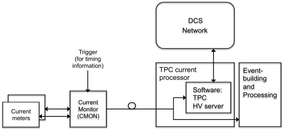
Figure 3.1: Schematic showing the control and monitoring of the GEM current system [3].
