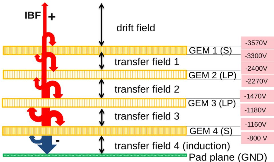
Figure 1.5: Representation of ion backflow on the four GEM foils together with the applied voltages at each foil [6].
