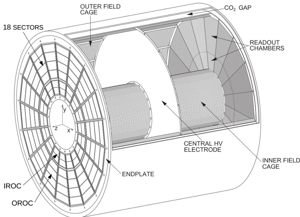
Figure 1.2: Schematic view of the ALICE Time Projection Chamber [3].
