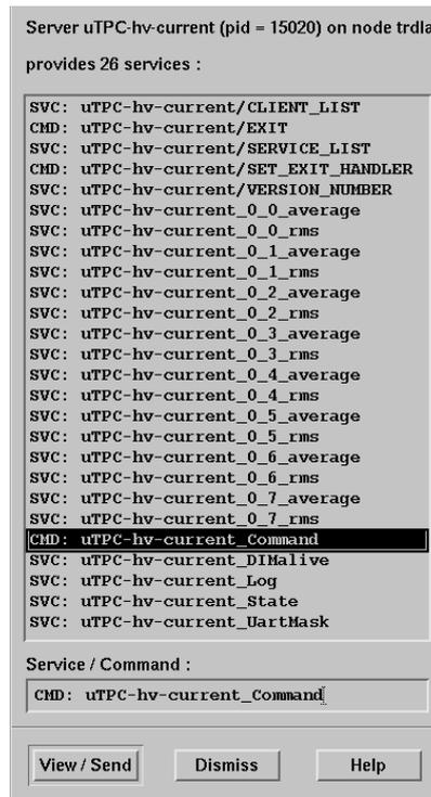
Figure 3.2: DIM client window with the available DIM services. The command service enables the control of the board via network.
