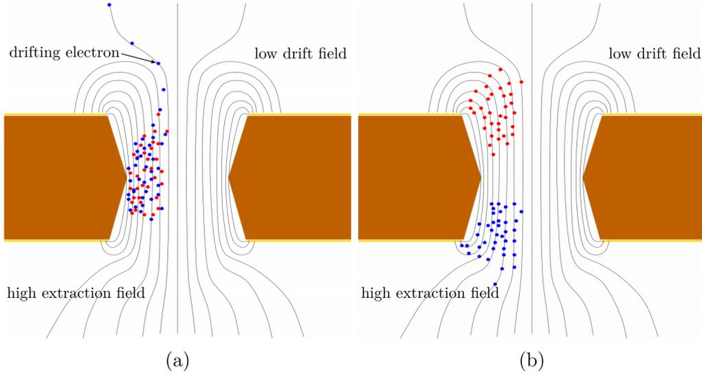
Figure 1.3: *Simulation of the Electric field at the GEM holes: (a) electrons (blue) are guided into the holes by the created field, where avalanches of electron-ion pairs are generated. (b) The asymmetric field configuration together with the small ion (red) mobility lead to efficient backflow suppression [4].*
