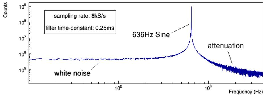
Figure 4.3: *Frequency spectrum of a filtered sine and white noise when a digital filter cut-off frequency of 636 Hz is applied.*
