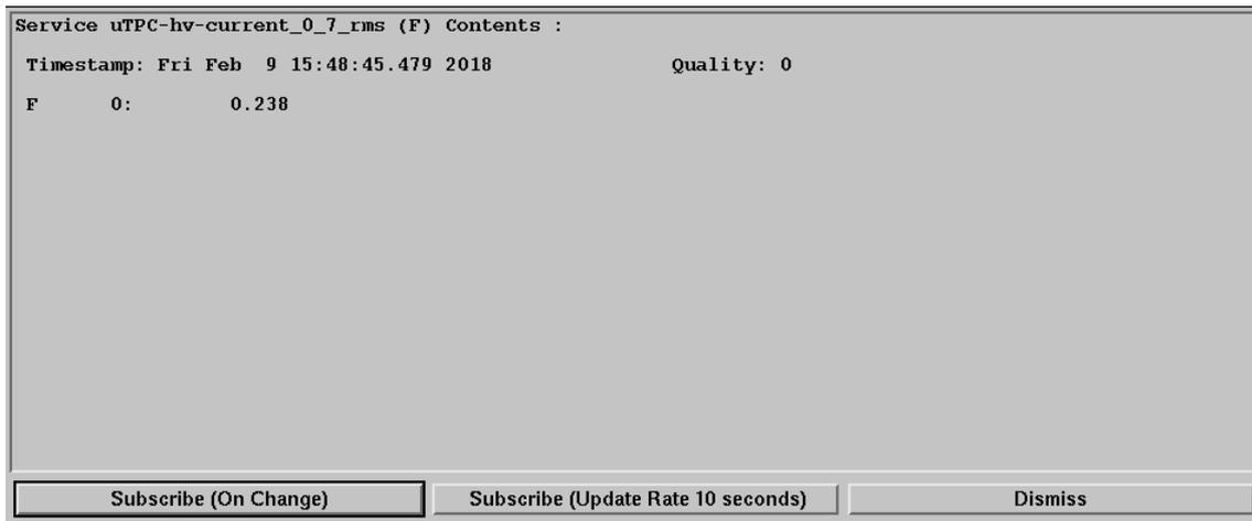
Figure 3.4: Example of the DIM client display showing the RMS value in nA units.
