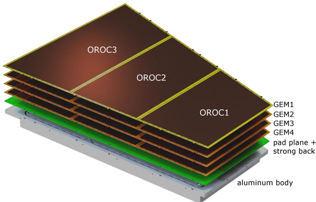
Figure 1.4: *Exploded view of the Outer Readout Chamber and its main components. The Inner Read Out Chamber consist, similarly of a single GEM stack [5].*
