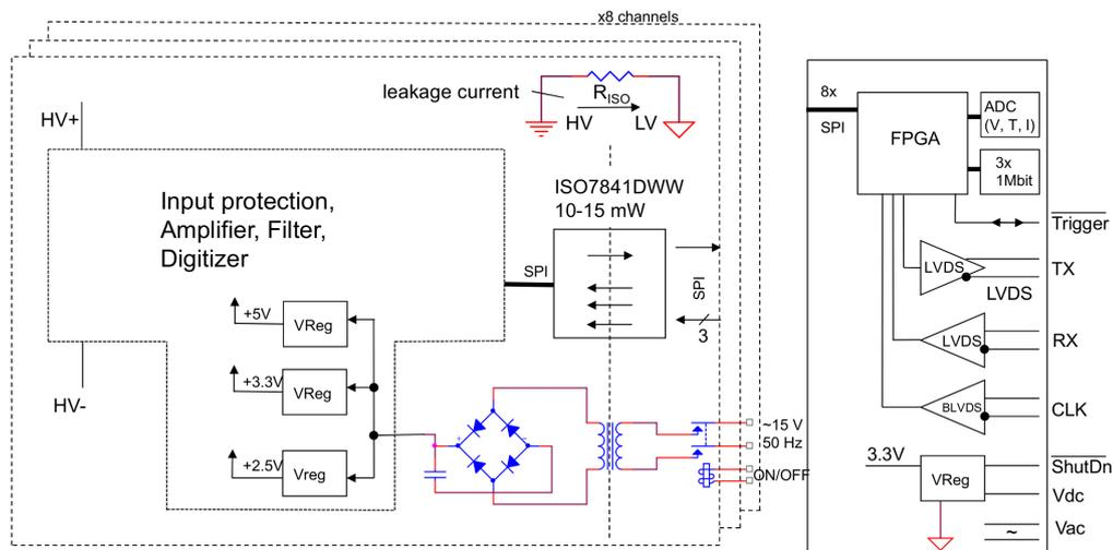
Figure 2.2: Block diagram of the front-end board [7].
