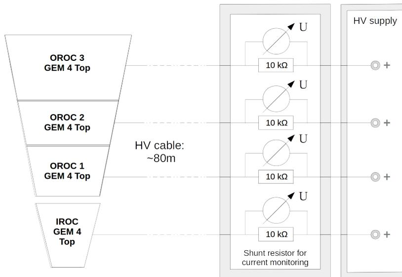
Figure 2.1: *GEM analogue current readout scheme.*
