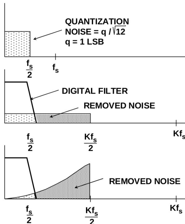
Figure 2.4:  $\Sigma$ - $\Delta$  modulation for quantization noise reduction. Oversampling, digital filtering, and noise shaping are the main filter operations [9].
