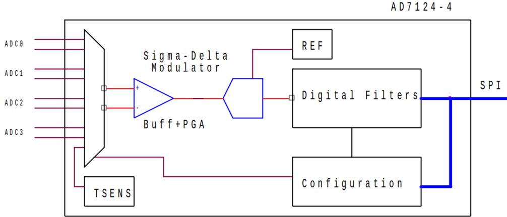
Figure 2.5: Block diagram of the AD7124-4 [7].
