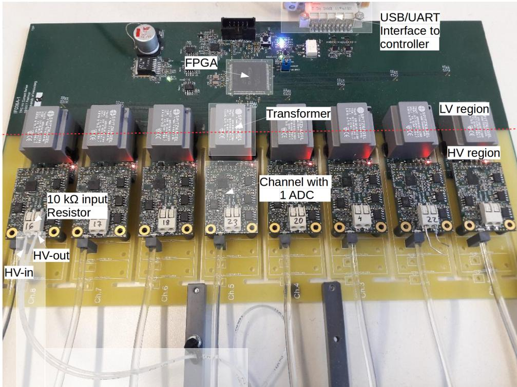
Figure 2.3: Readout board at the Physikalisches Institut and its main components. Its dimensions are: 17x28 cm
