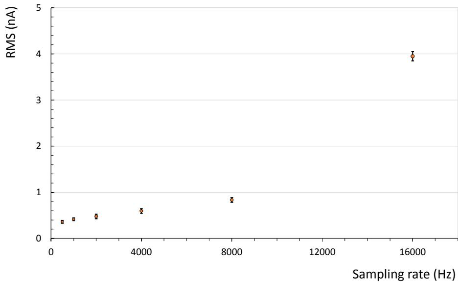
Figure 4.6: RMS values for the different sampling rates. The ADC noise is increasing for higher sampling rates.
