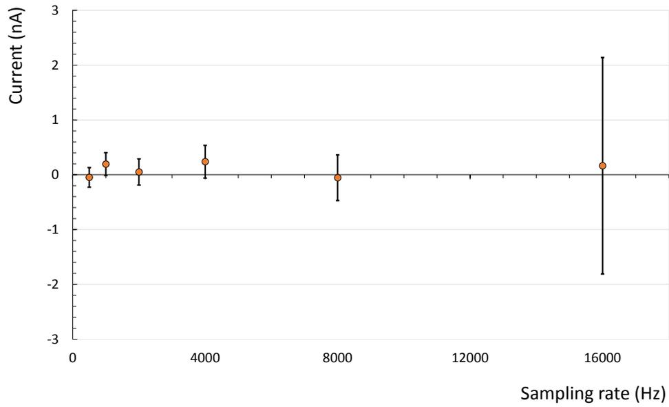
Figure 4.5: ADC operation noise for the different possible sampling rates. Dots indicate the mean value at no input and the vertical bars represent the RMS values.
