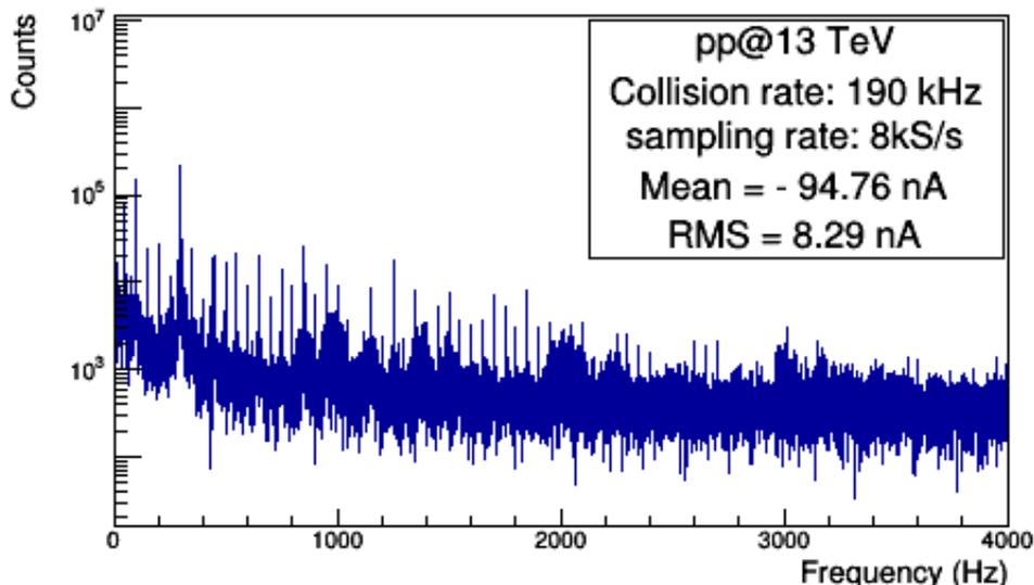
Figure 4.7: *Fourier Transformation of GEM current raw data acquired at ALICE during proton-proton collisions. The current was found to be  $(-95 \pm 8)$  nA.*
