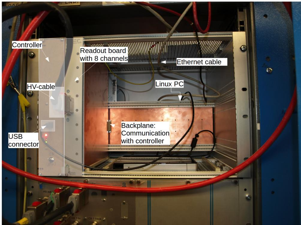
Figure 3.5: *GEM current readout system at Counting Room 4 and its main components.*
