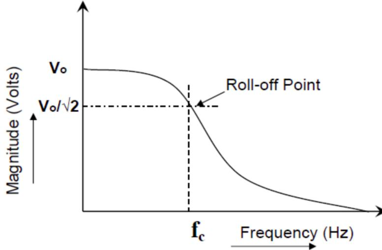
Figure 4.2: Frequency response of the RC low-pass filter. At the cut-off frequency  $f_c$ , the value of  $V_{out}$  has decreased by a factor of  $\sqrt{2}$  of its maximum [16].
