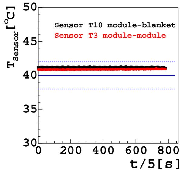
**Figure 4:** Horizontal Test: Time stability of the temperatures. The black points show the time behavior of a sensor between blanket and module ( $y=3\text{m}$ ), while the red points show the time behavior of a sensor in the air gap ( $y=2\text{m}$ ).
