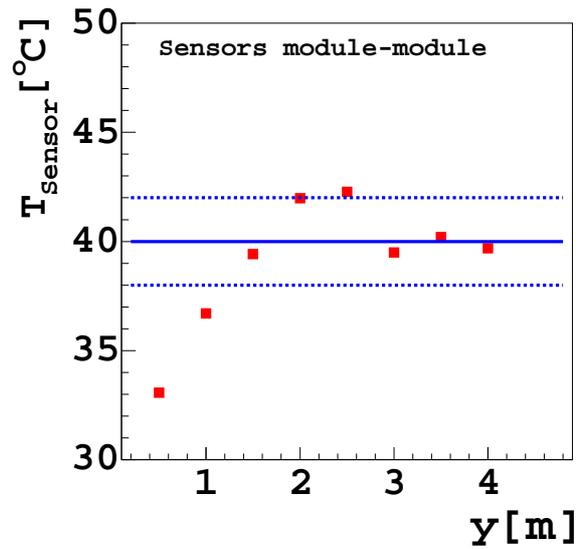
Figure 15: The  $T$ -profile along the vertical gap between the two rows of modules for a heating blanket steered with **two heating areas**.
