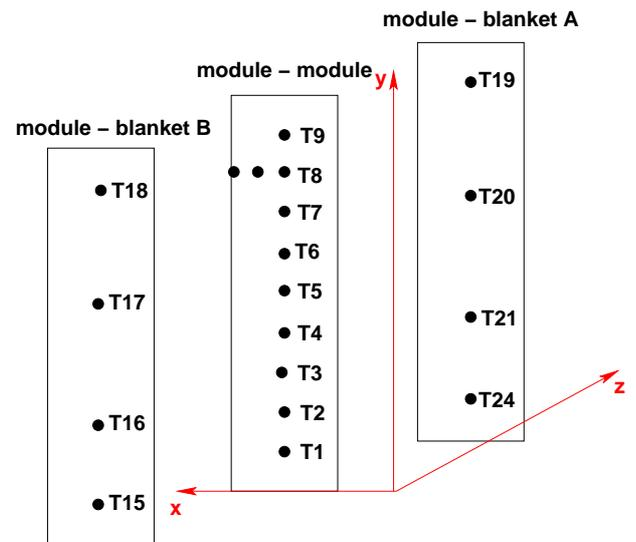
**Figure 7: Temperature sensors setup.**
