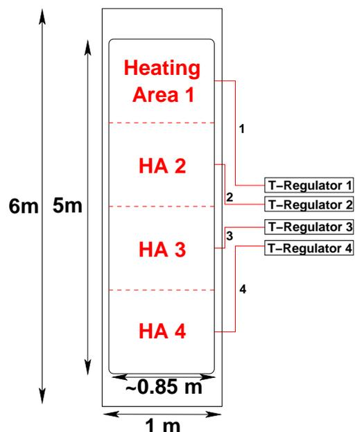
Figure 1: Schematic view of a heating blanket. The label 'HA' stands for 'heating area'.
