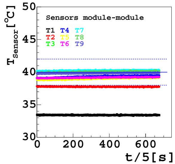
Figure 11: Time stability of the temperatures between the two rows of modules.
