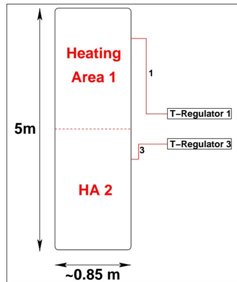
Figure 13: Schematic view of heating blanket steered with two heating areas.
