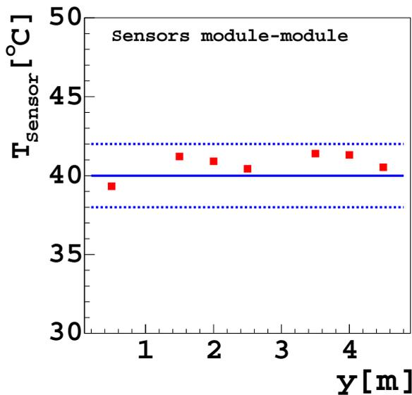
**Figure 3:** Horizontal Test: Temperatures in the air gap between the modules after reaching thermal equilibrium. The x-axis gives the sensor position along the modules. All temperatures lie within the  $\pm 2^\circ\text{C}$  band around the nominal value of  $40^\circ\text{C}$ .
