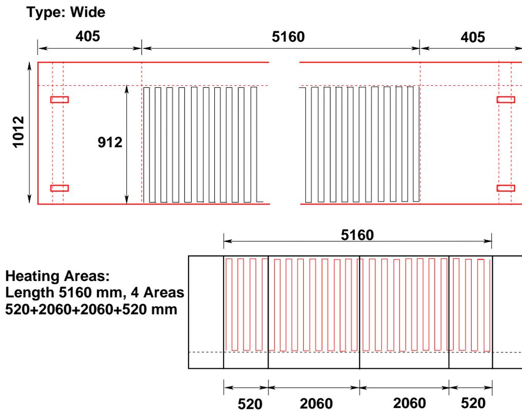
Figure 17: Schematic view of the revised design of the heating blanket.
