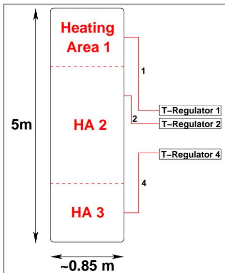
Figure 12: Schematic view of heating blanket steered with three heating areas.
