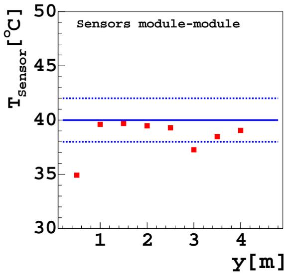
Figure 14: The  $T$ -profile along the vertical gap between the two rows of modules for a heating blanket steered with **three heating areas**.
