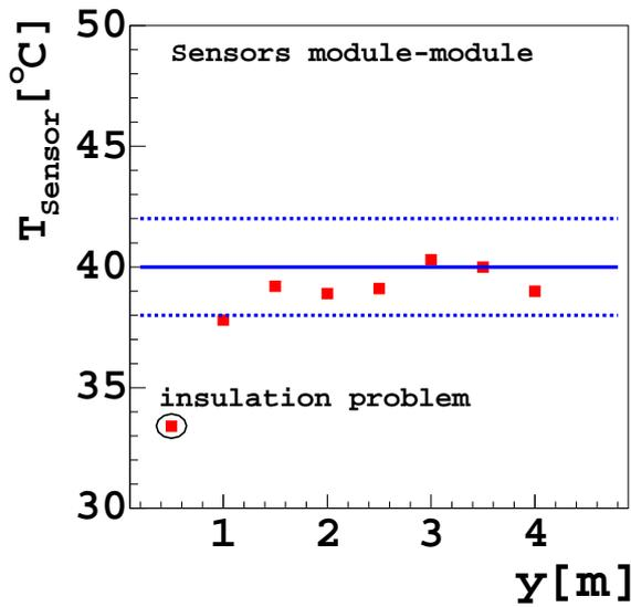
Figure 10: The T-profile along the vertical gap between the two rows of modules.
