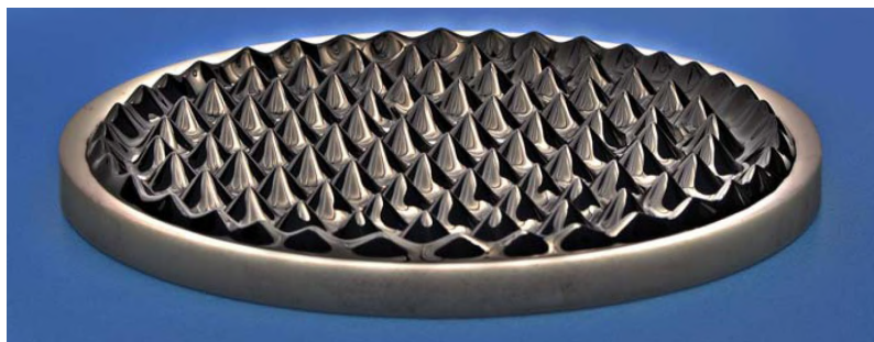
Figure 2.7: The Rosensweig instability in a ferrofluid (taken from Holger Knieling et. al [37]).
