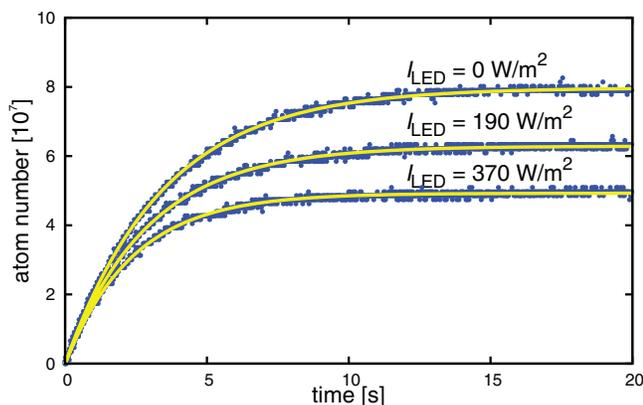
FIG. 4. Loading curve of MOT with and without the LED. The data points correspond to the fluorescence signal converted into a total number of trapped atoms. The yellow solid lines are a fit of Eq. (1). The intensity of the LED are  $I_{\text{LED}} = 190 \text{ W/m}^2$  and  $I_{\text{LED}} = 370 \text{ W/m}^2$ , measured at the position of the atom cloud.
