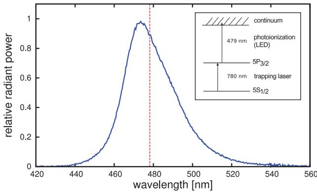
FIG. 1. Spectrum of the LED. The red dotted line indicates the ionization threshold of Rb atoms in the first excited  $5P_{3/2}$  state. Inset: Level scheme of  $^{85}\text{Rb}$ .
