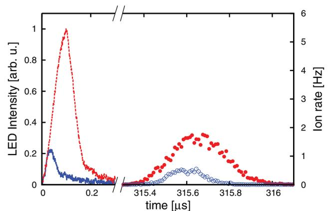
FIG. 5. Measurement of temporal intensity distributions of the LED in pulsed mode. The LED is pulsed for 30 ns (blue solid curve) or 100 ns (red dashed curve). After a time of flight of 315  $\mu\text{s}$  the ions are detected and have a time spread of 190 ns (blue open circles) and 300 ns (red solid circles) (FWHM), respectively.
