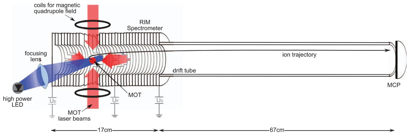
FIG. 3. Schematics of the experimental setup. Rb atoms are trapped in a magneto-optical trap in the center of a recoil-ion momentum spectrometer and ionized by the light emitted from the LED, which is imaged onto the atom cloud. The aspherical imaging lens has a focal length  $f = 40$  mm. The ions are accelerated towards the MCP detector by the voltage  $U_E$  and focused in time by the voltage  $U_F$  before entering the field free drift region with the voltage  $U_D = 0$ .
