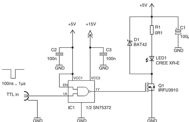
FIG. 2. Circuit diagram of the pulsed LED. For explanation see text.
