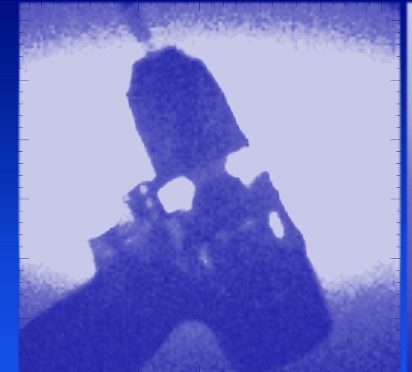
radiography of a cordless screwdriver
