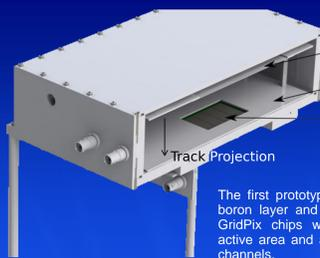
The first prototype consists of a one boron layer and a readout unit of 8 GridPix chips with approx. 15 cm<sup>2</sup> active area and approx. 460000 pixel channels.
