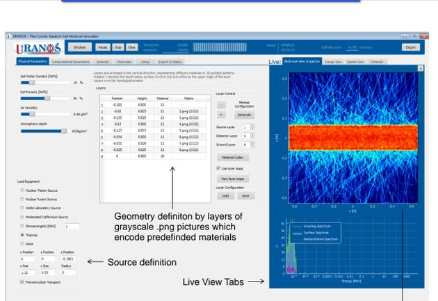
Geometry definition by layers of grayscale .png pictures which encode predefined materials
