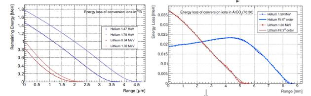
Conversion ion energy spectra for boron layers from 100 nm up to 2500 nm thickness in steps of 200 nm. The higher escape energies correspond to the helium ions whereas the lower correspond to the lithium ions.
