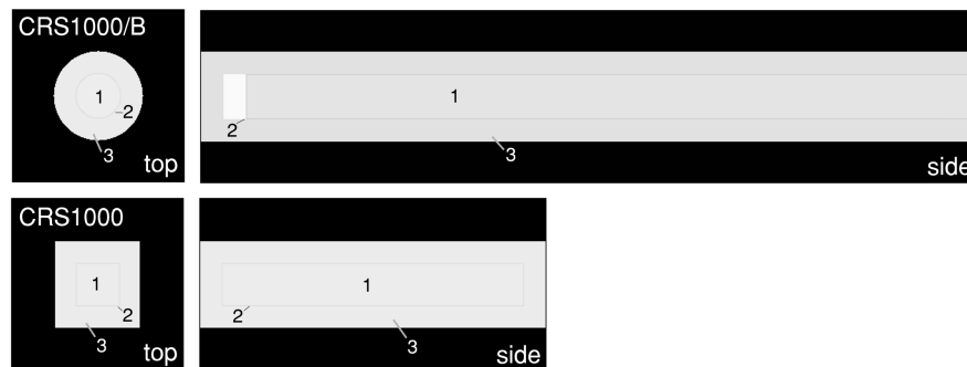
Figure 89: Cross sections of the detector models for the CRS1000 (bottom) and 1000/B (top) detectors with their proportional counter tube (1) in a stainless steel housing (2), surrounded by a polyethylene moderator. The grayscale pictures are the actual geometry input files.
