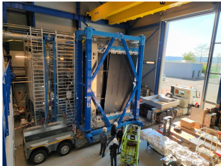
The first four frames are loaded in a transport cage in the assembly hall at Point 8, May 3, 2021. Photo by Sune Jakobsen..
