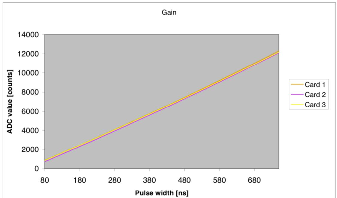
If a regular curve fit is made (linear regression), the equations of the three sub-modules are approximately the same. The main difference is the offset of the curve (which can be adjusted with an external potentiometer), the gain is the same. The linearity of the curve is not so bad, because for all the curves the coefficient of determination ( $R^2$ ) is approximately 0.999.
