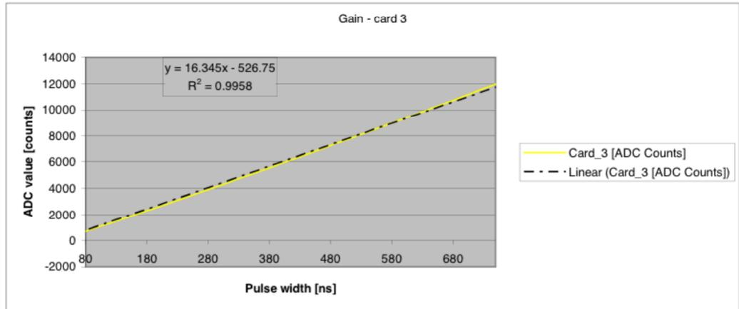
In the next tables are shown the gain for the two measurements and the error for each gain respect to the mean gain in % ( mean value – gain / mean value x 100).
