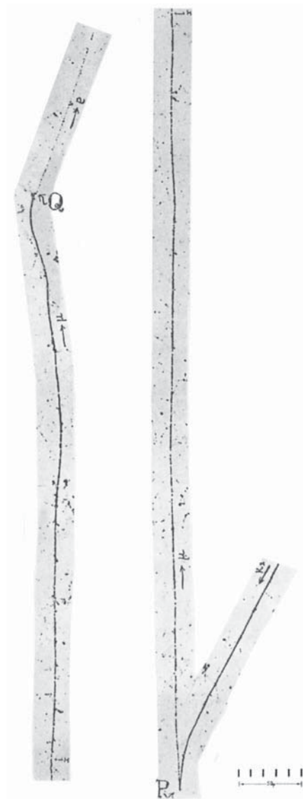
Figure 3.1. A \kappa ( K ) meson stops at P , decaying into a muon and neutrals. The muon decays at Q to an electron and neutrals. The muon track is shown in two long sections. Note the lighter ionization produced by the electron, contrasted with the heavy ionization produced by the muon near the end of its range. The mass of the \kappa was measured by scattering and grain density to be 562 \pm 70 MeV (Ref. 3.4).
