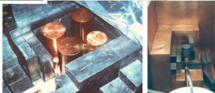
Fig. 1. The HEIDELBERG–MOSCOW \beta\beta -experiment in the Gran Sasso (top), and four of the enriched detectors during installation (bottom left). The fifth detector was installed in an extra shielding using electrolytic copper as inner shield (bottom right).
