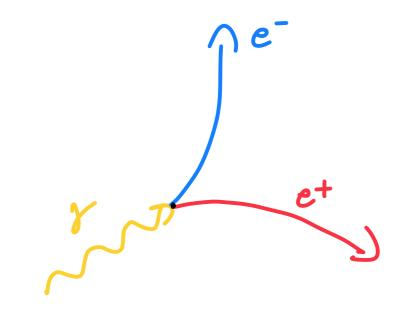
Photon can convert into an electron positron pair once its close to some nucleus (energy-momentum conservation)
