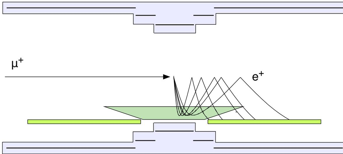
Gradient field gives constant bending radius independent of angle
