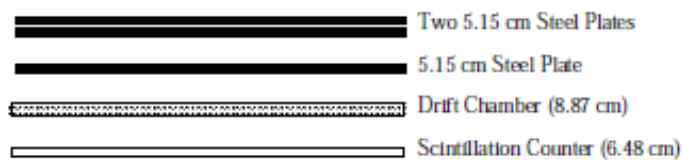
Figure 2.6: Stack layout of a CCFR target cart. A drift chamber is positioned after every two steel plates and a scintillation counter is found after every four.
