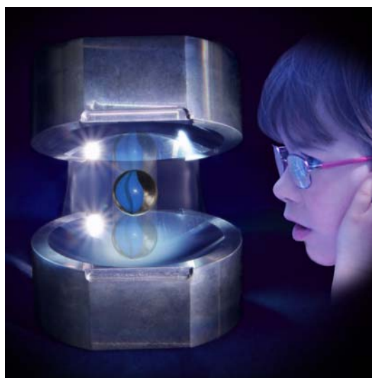
Figure caption: Microwave photons trapped between superconducting mirrors are counted without being destroyed.
