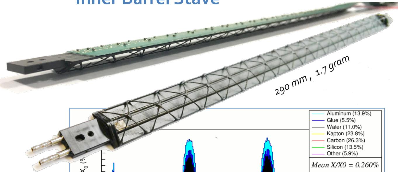
Silicon sensor + readout circuitry
