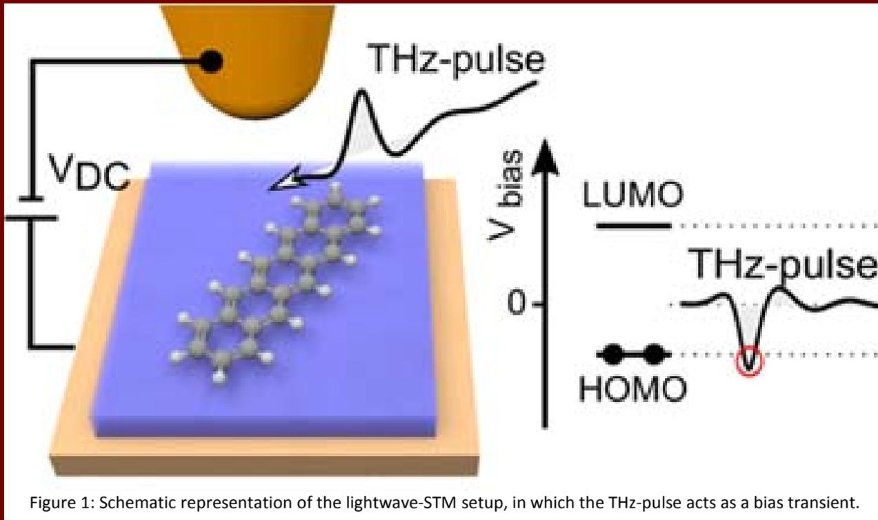
Figure 1: Schematic representation of the lightwave-STM setup, in which the THz-pulse acts as a bias transient.
