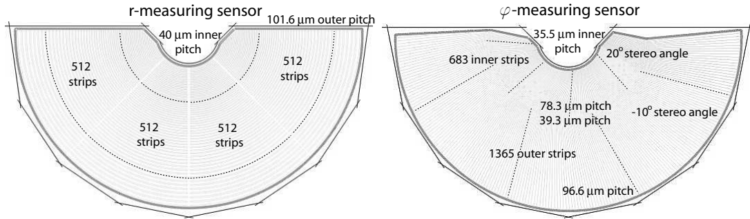
Figure 2.5: The two types of measuring sensors used in the Vertex Locator. (Figure from [5].)
