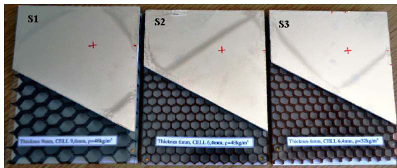
Figure 10.11: Carbon fibre honeycomb plates of different size between two Rohacell plates.
