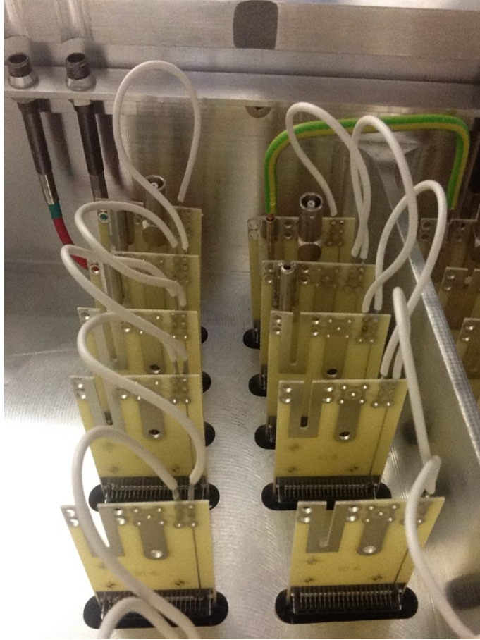
Figure 4.7: Shorting cards, on the backside of the chamber body, connecting all pads of the OROC. The cable in green and yellow connects two rows with each other. The red cables in the back are the HV inputs for the GEMs.
