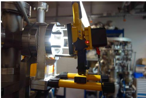
(c) Placement of light source in front of opened valve (component 1).
