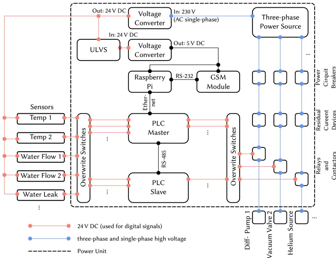
Figure 4: Implementation and connections of hardware components inside power unit. Some details such as safety fuses and power supply for PLCs and for the override switches have been omitted for a more concise representation. For the complete circuit layout please see appendix D.
