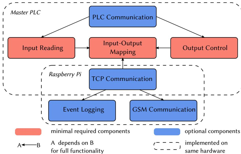
Figure 13: Overview of modules required for a working power unit control.
