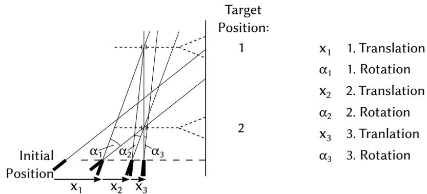
Figure 24: Representation of step 10 to 16 of alignment of the telescope axis to the detector translation rails axis. The enumeration on the right shows the necessary movement order. The translation  $x_3$  shows the slight overshoot necessary to perfectly center the view axis in the last orientation change  $\alpha_3$ .
