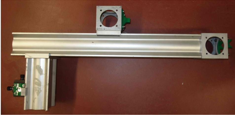
Figure 23: Target for aligning telescope view axis in parallel to linear rails. Green protrusions at the middle and end are the contact points for the linear rails. The target center can be adjusted with a movable aperture seen in the lower left corner.
