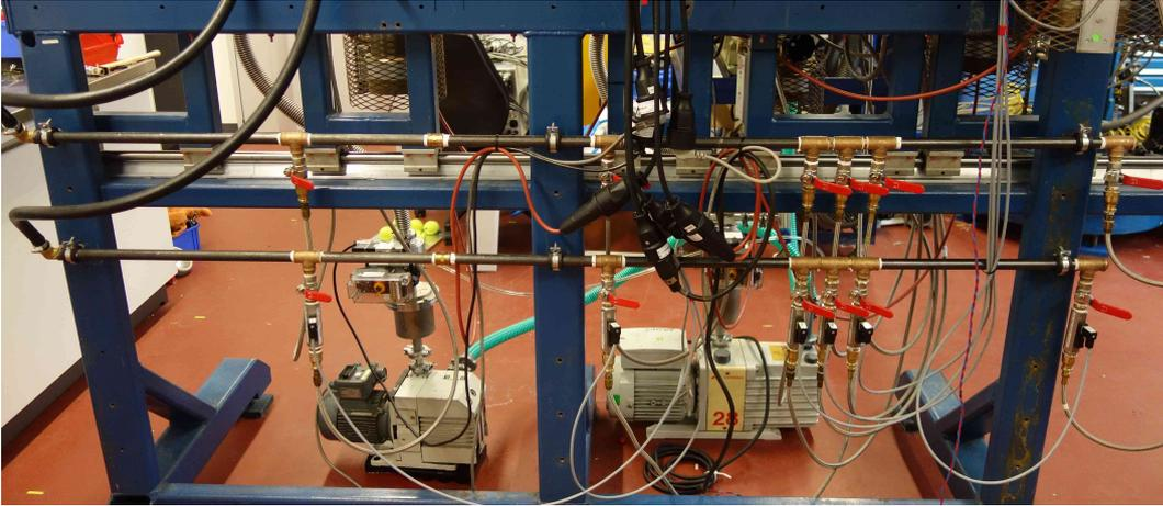
Figure 20: Cooling system for the ToF arm. Inlet is connected to the upper pipe and the outlet affixed to the lower pipe. Solenoid and check valves as well as pressure regulator are attached at the ceiling and not pictured here.
