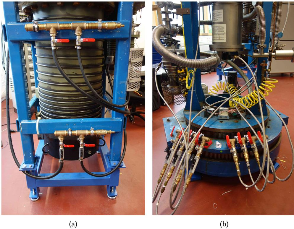
Figure 21: Cooling system for source chamber (a) and scattering chamber (b). System for source chamber was built in ?. The main connections for in- and outlets are not attached.
