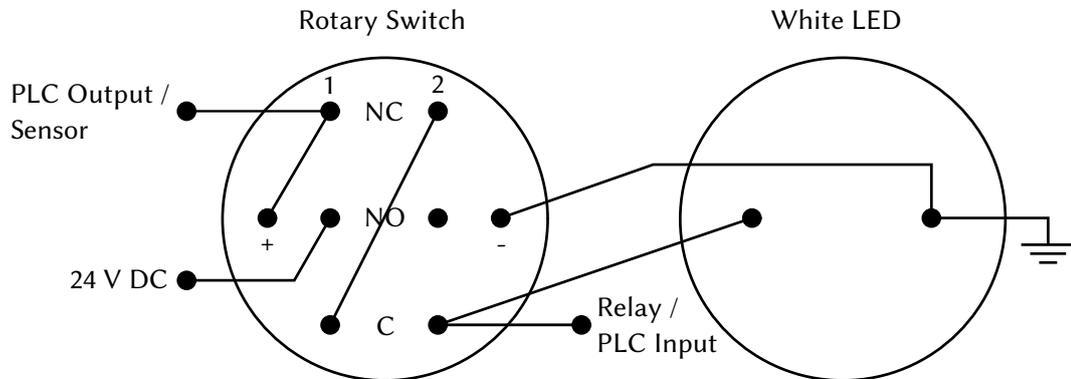
Figure 7: Backside connections of the rotary switch. Input and Output schematics are similar except for different connections on NC1 and C2. The switch consists of two separate two-way-levers (labeled with 1 and 2) which are interconnected between NC and C. The external LED has no predefined polarity since it uses a built-in rectifier.
