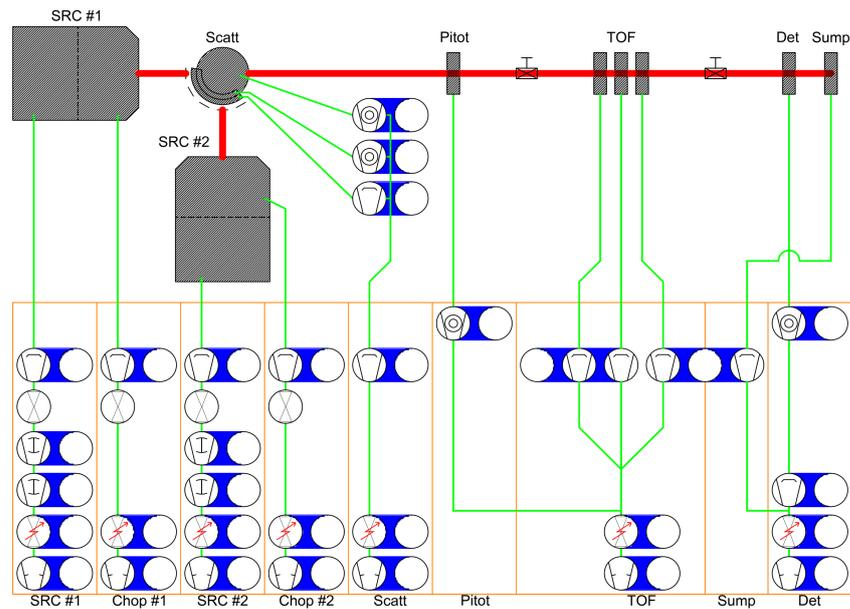
Figure 10: Layout of predefined outputs on the front panel of the power unit. The position of the electrical consumers in this layout corresponds to the position of their respective LED-switch pairs on the right hand side front panel. Designed by Tom Turczyk, permission to publish given on 06.05.2020
