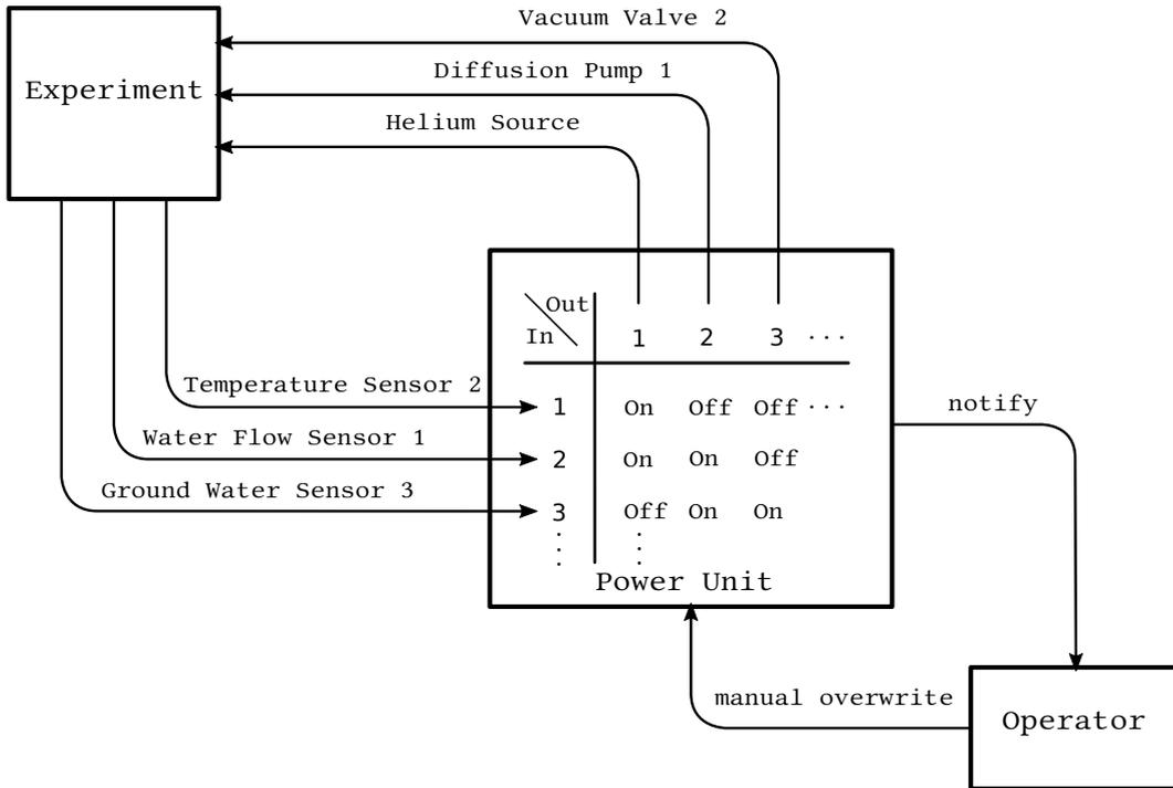
Figure 3: Control logic of power unit. A predefined matrix decides which outputs are disabled if a certain input registers a value which is different from its expected value.
