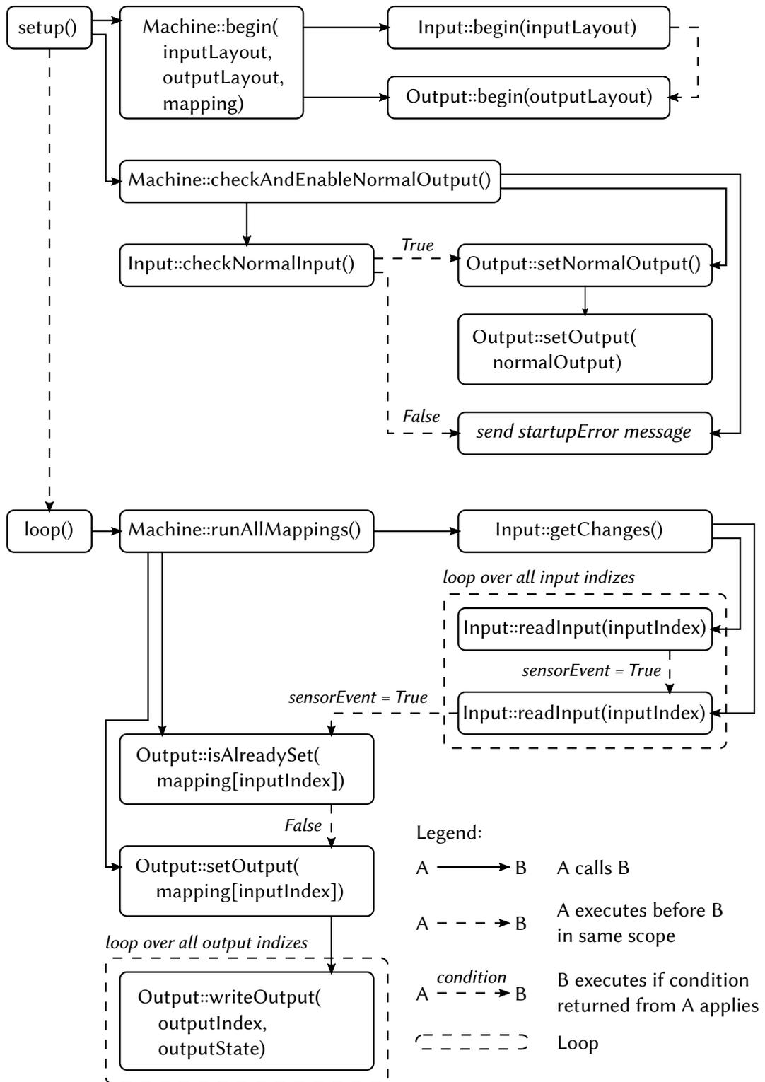
Figure 15: Call and execution structure of the mapping logic within the master PLC. Logging and communication function calls are omitted.
