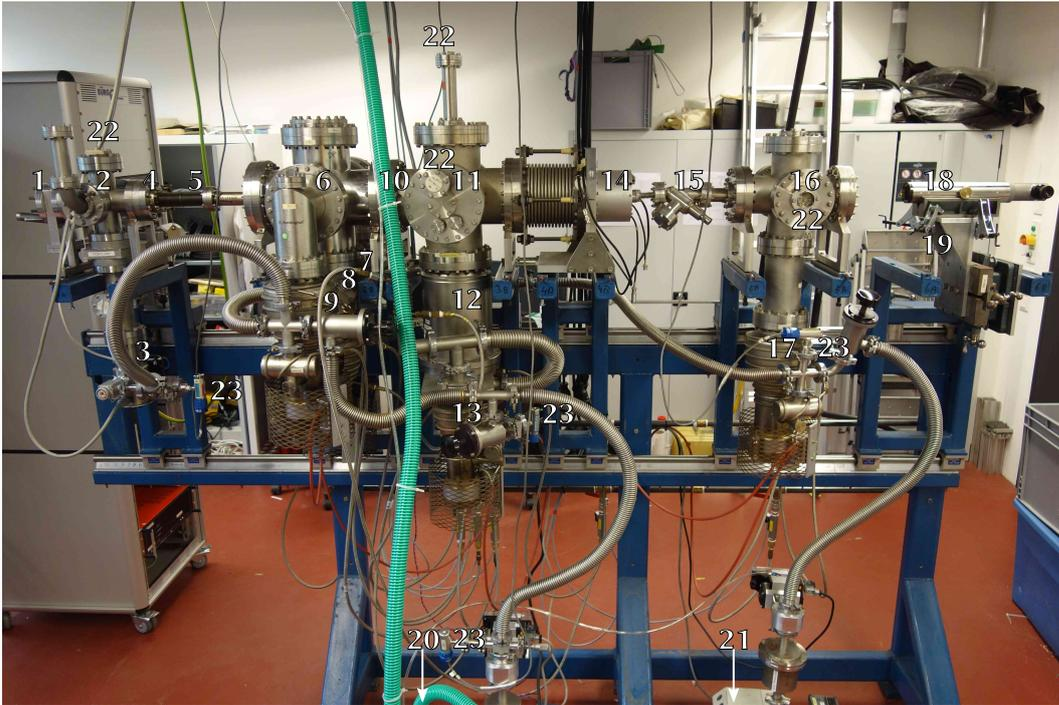
Figure 31: time-of-flight detector chamber in its completed state. Enumerations refer to table 6. In addition, label 22 annotates ionization pressure gauges and label 23 indicates fore-vacuum pressure gauges.
