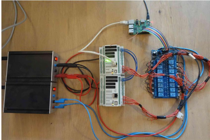
Figure 11: Test bench to simulate inputs for master and slave PLC. From left to right: Power sources (black), master (upper) and slave (lower) PLC, Raspberry Pi (green), Relayboard (blue).
