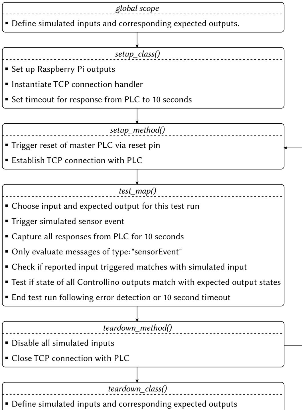
Figure 12: Flow chart of the test bench software. Arrows indicate the execution order. The tasks of each method are listed below its name. The related scripts can be found in appendix C.
