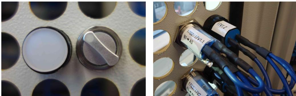
Figure 8: Front and back view of rotary switch and status LED. Currently in "automatic" setting. Each component is labeled with a reference from the circuit diagram in section D.
