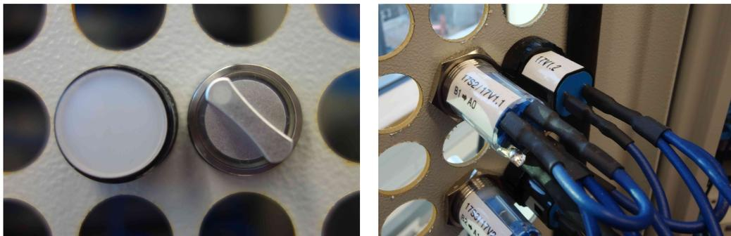
Figure 8: Front and back view of rotary switch and status LED. Currently in "automatic" setting. Each component is labeled with a reference from the circuit diagram in section D.
