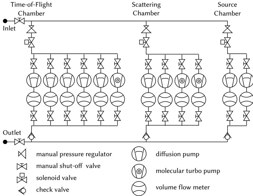
Figure 19: Schematics of the cooling system for GI-HAS experiment. Initial concept was designed by Schko Sabir as part of his master thesis but was not published there. Solenoid valves are operated by power unit. The three joint in and outlets of the chambers come down from the laboratory ceiling.
