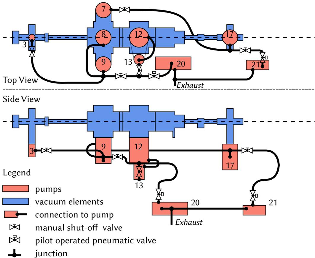
Figure 17: Fore-vacuum configuration for all ToF arm vacuum pumps. Support structure is not shown for conciseness. Annotations can be found in table 6.
