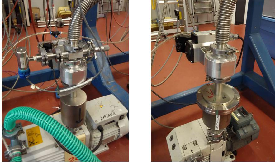
(a) Pump: *Edwards E2M28* (20 of table 6) (b) Pump: *Trivac D4B 112 45* (21 of table 6)
