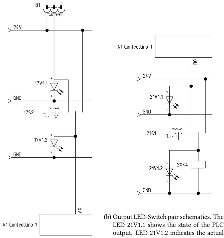
(a) Input LED-Switch pair schematics. The LED 17V1.1 shows the state of the sensor output. LED 17V1.2 indicates the actual state of the corresponding PLC input. Automatic setting means state of sensor gets passed on to PLC.
