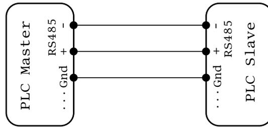
Figure 14: Wiring schematics for RS-485 connection between two Controllino Mega.
