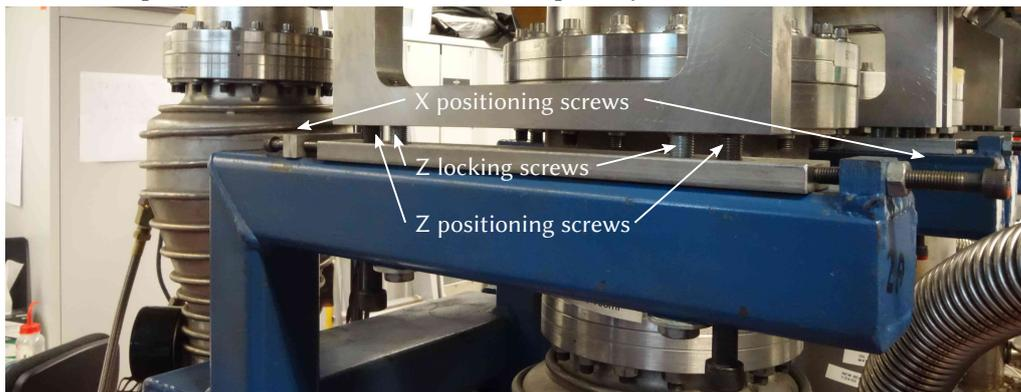
(e) Z and X positioning screws. Each frame has two adjustable mount points.
