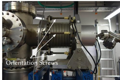
(d) Detector with 4 orientation screws. Placed point symmetrical around view axis.
