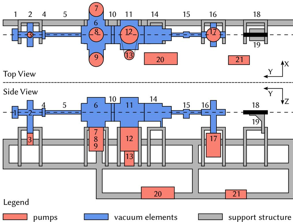
Figure 16: Time-of-Flight detector chamber. The scattering chamber connects to the left hand side. A telescope (black) is used to define and align the beam axis. Annotations can be found in table 6.
