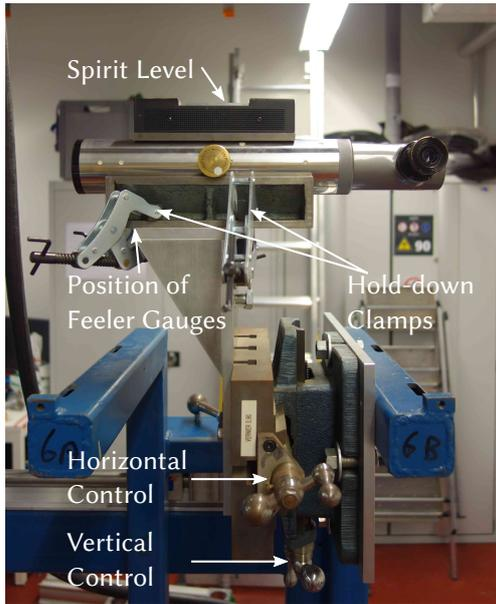
(a) Telescope mount and positioning
