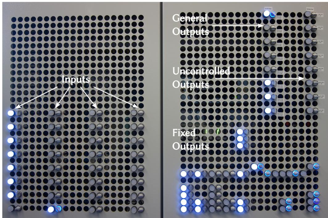
Figure 29: Front cover of the power unit. Each rotary switch has an internal blue LED indicating the state if automatic mode was chosen. White external LED shows the actual state. Horizontal position means: off, diagonal: automatic, vertical: on.
