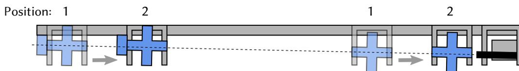
Figure 22: Illustration of alignment issue. The chosen beam line has to be parallel to the movement of the detector. The vacuum components are aligned to the view axis of the telescope (black box) in position 1. Their central axis moves away from the previously defined beam line, if it is not parallel to the linear rail. For conciseness only the first and last vacuum component is shown. Not to scale.
