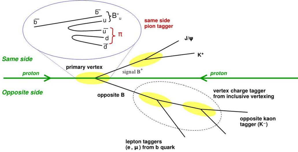
Figure 3.9: Tagging process at the LHCb experiment [22].
