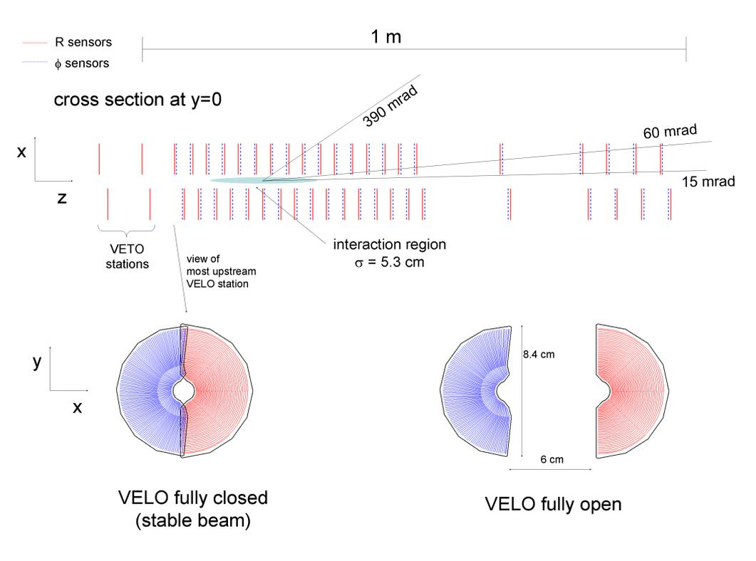
**Figure 3.5:** Schematical overview of the placement of the Vertex Locator along the beam axis. The subsensors of each station can be opened during beam injection [20].
