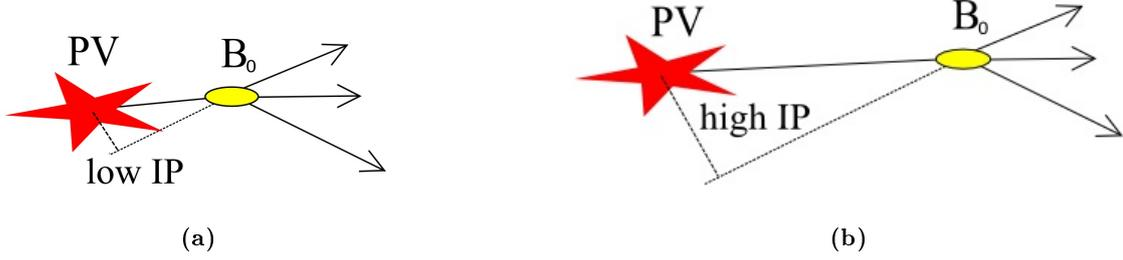
**Figure 6.4:** Particles originating from short-lived  $B^0$  mesons (a) have in general lower impact parameters than for long-lived  $B^0$  mesons (b). A cut on the impact parameter thus removes short-lived  $B^0$  and introduces a bias of the measured decay time.
