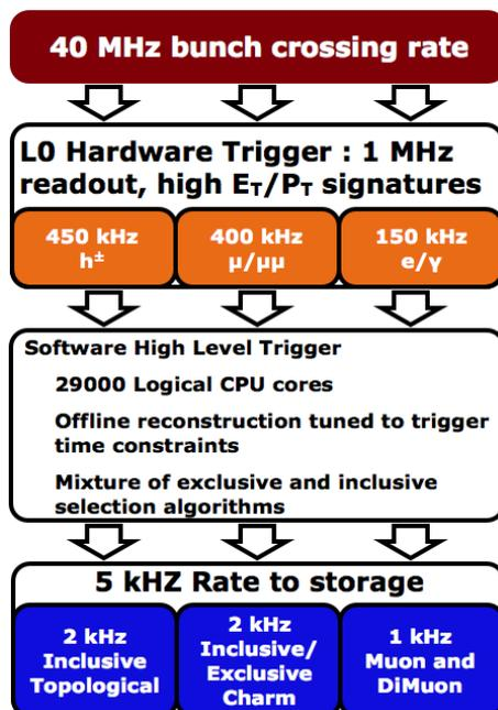
Figure 3.8: Schematic overview of the LHCb trigger structure [17].
