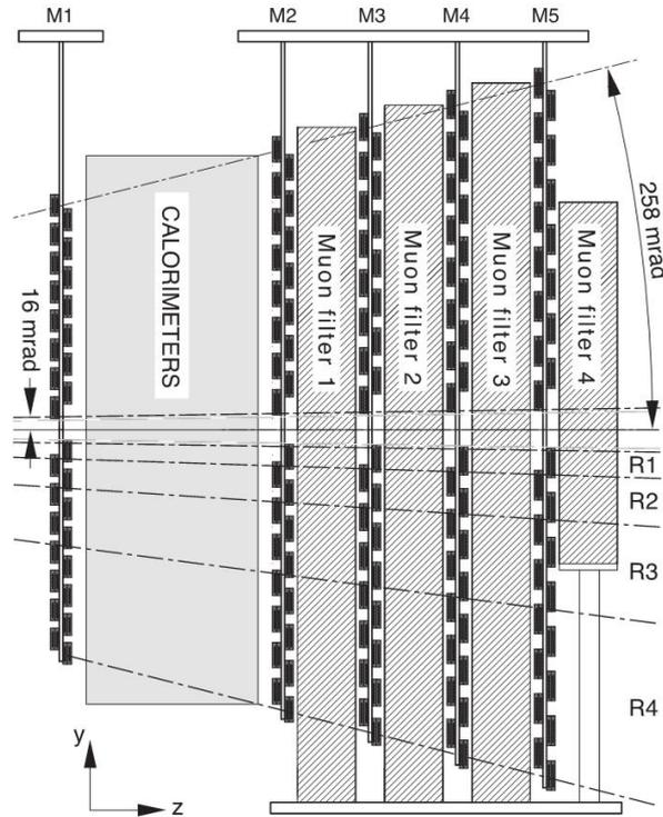
Figure 3.7: Schematic overview of the LHCb muon system [20].
