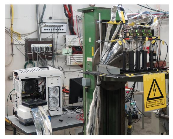
FIGURE 8.3: The DESY testbeam setup: On the top right, the telescope, mounted on a movable stage, provided by the DESY testbeam group. The telescope is connected to the RO computer via 4 m long shielded ribbon cables.
