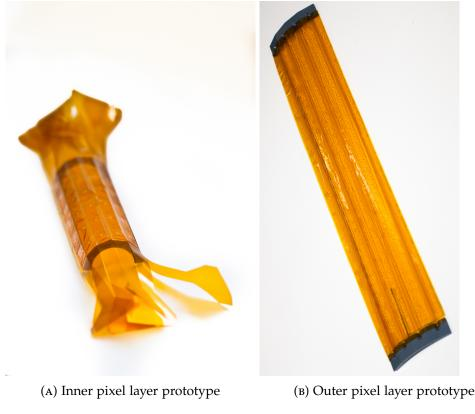
FIGURE 2.5: Kapton pixel support structure prototypes
