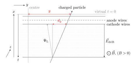
Figure 4.12: Tracklet reconstruction and correction: The primary ionization electrons from a traversing charged particle are deflected by the Lorentz angle  $\Psi_{\rm L}$ . This results in an offset of the apparent deflection which is corrected. The y position with respect to the chamber centre holds for the virtual t = 0 radial position.
