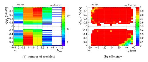
Figure 4.16: Tracklet efficiencies in Monte Carlo. Left: The number of tracklets found per expected one (from Monte Carlo track references) clearly shows that tracklets are found multiple times. Right: The efficiency slightly depends on the transverse position and the transverse momentum.
