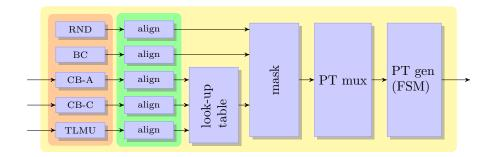
Figure 4.4: Overview of CB-B: The central processing unit receives the trigger contributions from different sources. Besides the sampled input signals, which can be delayed to accommodate for different latencies, random (RND) and BC-derived signals are used. The inputs from T0, V0, and TOF are fed into a look-up table. The final trigger output is generated in a state machine reflecting the FEE.
