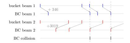
Figure 3.2: LHC filling scheme and resulting collisions: The filled RF buckets are shown for the two beams. A given bucket passes the ALICE interaction point at a certain value of the Bunch Crossing counter (BC). A collision occurs if two bunches pass at the same time.
