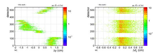
Figure 4.18: Shifts of tracklets with respect to Monte Carlo truth for different detector chambers. The gaps correspond to super-modules which were not yet installed in Run 1. Left: The shift distribution for the transverse position y. Right: The shift distribution for the deflection.
