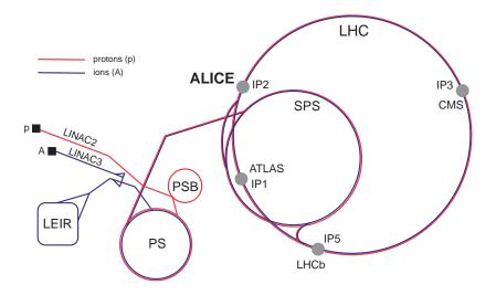
Figure 3.1: LHC injector chain and interaction points: The LHC requires a set of preaccelerators to reach the injection energy of 450 GeV. The opposing beams intersect in four interaction points which are equipped with experiments.
