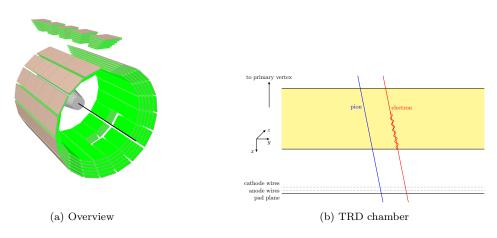
Figure 3.4: Overview of the TRD installation. Left: The TRD consists of 6 layers of tracking chambers and is segmented into 18 sectors in azimuth with 5 stacks in longitudinal direction each. The picture shows the full installation with the holes in front of PHOS for three super-modules. Right: The cross-sectional view of one TRD chamber shows the radiator, the drift region separated by the cathode wires from the amplification region.
