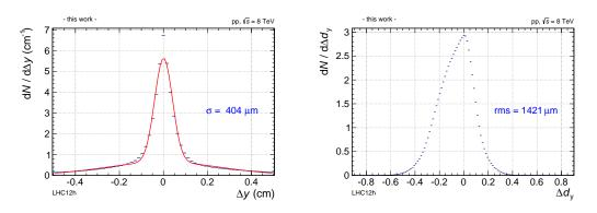
Figure 4.19: Tracklet residuals in y and  $d_y$ : The residuals are extracted from the comparison to a helix fit through the tracklets from GTU tracks. The correction on  $d_y$  for the Lorentz drift in the magnetic field is negative here.
