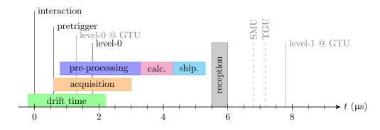
Figure 4.2: Trigger timing relative to the interaction. All FEE timings are determined by the pretrigger and configured with respect to it. The latency of the pretrigger determines the position of the sampling window (green). The acquisition (orange) of the delayed signals starts with the pretrigger. The pre-processing (blue), tracklet calculation (magenta), and tracklet shipping (cyan) start with a small offset. The GTU-related timings are shown in grey.
