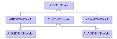
Figure 4.14: TRD online tracking class hierarchy: The abstract base classes AliVTrdTrack and AliVTrdTracklet provide the interface to the TRD online tracking information for the use in analyses. The realizations in ESDs and AODs vary in the level of detail.
