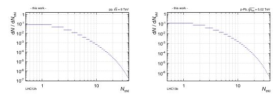
Figure 4.20: Tracklet multiplicities per chamber as observed in pp collisions at  $\sqrt{s} = 8$  TeV (left) and p–Pb collisions at  $\sqrt{s_{\text{NN}}} = 5.023$  TeV (right). The values are low enough for the online tracking to finish in time for the trigger contribution.
