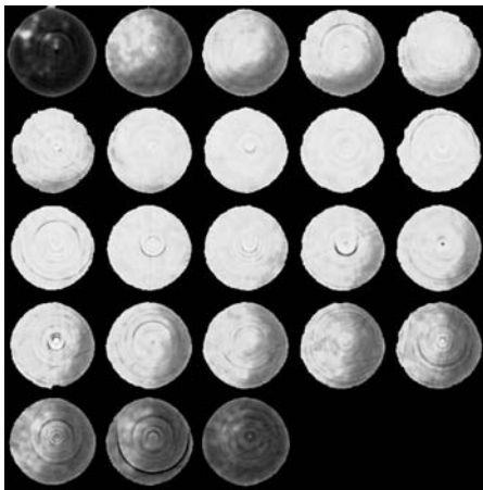
Figure 3.30: Diffusion of water in sand. Top view. Slices of the reconstructed water distribution. The top layer is the upper left image. The bottom layer is shown in the middle of the last row.
