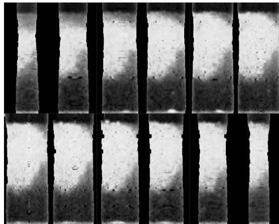
Figure 3.31: Diffusion of water in sand. Side View. Shown are vertical layers of the reconstructed distribution. Areas containing parts of the surrounding plastic tube have been cut away.
