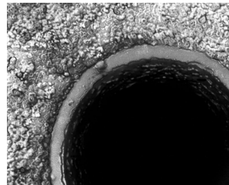
Figure 68: Microscope image with focus stacking: hole of a boron-coated GEM.
