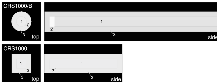
Figure 169: Cross sections of the detector models for the CRS1000 (bottom) and 1000/B (top) detectors with their proportional counter tube (1) in a stainless steel housing (2), surrounded by a polyethylene moderator. The grayscale pictures are the actual geometry input files.
