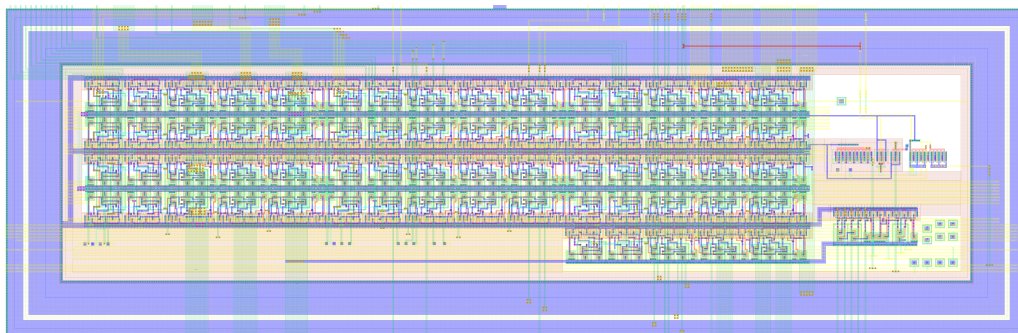
Figure 10.6: Layout of the radiation hard EoC of the HitPix with a size of 200 \mu\text{m} \times 64 \mu\text{m} .
