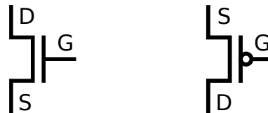
Figure 1.8: symbol for NMOS ( left ) and PMOS ( right ). Well contacts are omitted as they are connected to GND / VDD.
