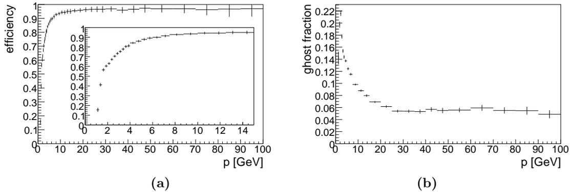
**Figure 3.5:** Reconstruction efficiency (a) and ghost fraction (b) for Long tracks found by the Forward Tracking against momentum.
