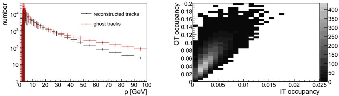
(a) This figure shows the total number of reconstructed particles and ghosts per momentum bin. It can be seen that the number of ghosts diminishes more slowly with momentum than the number of particles. (Note the logarithmic scale.)
