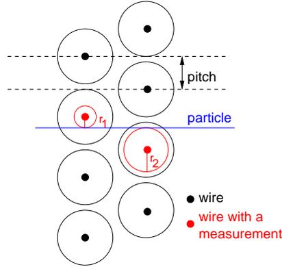
**Figure 5.8:** *The figure shows a cluster produced for a particle incident perpendicular to the detector layer. The amount of staggering between the two monolayers is called the pitch.*
