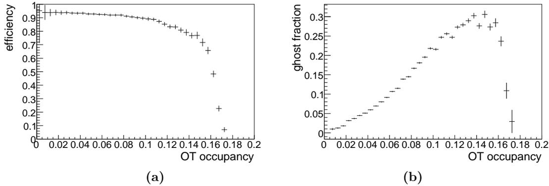
**Figure 3.9:** Reconstruction efficiency (a) and ghost fraction (b) for  $T$  tracks found by the  $T$  station seeding against OT occupancy. Both curves drop at high occupancy because of cuts applied in the algorithm (see text).
