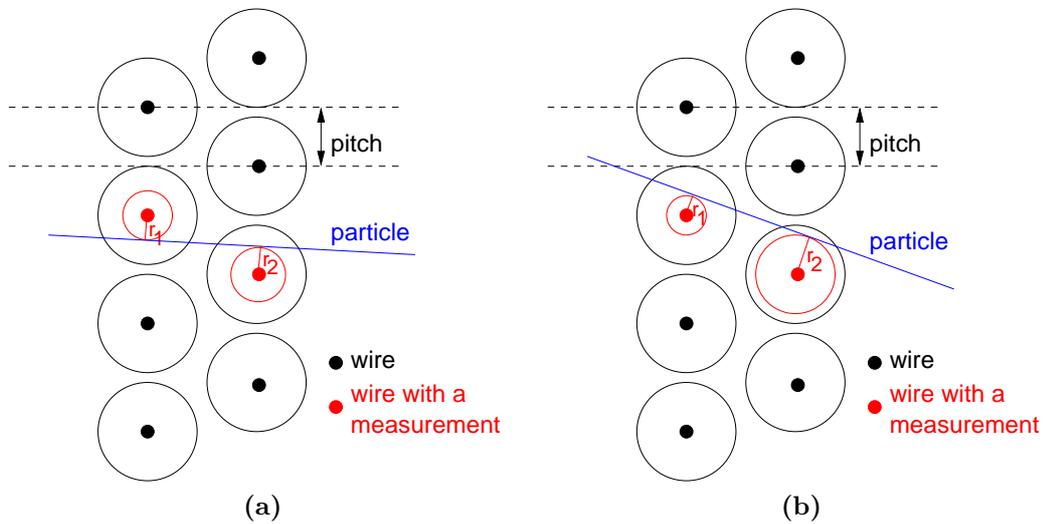
**Figure 5.10:** For particles passing through the detector with a non-vanishing slope, there are two situations: the particle passes either between the two wires (a), or it does not (b).
