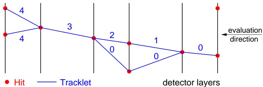
**Figure 4.4:** Sketch of the state of the automaton after the evolution phase: tracklet counters are shown next to each tracklet; the neighbourhood relation itself is not shown because it would needlessly obscure the picture. The two tracklets which have a counter of zero do not have neighbours due to the large kink angles, therefore, their counter is never incremented.
