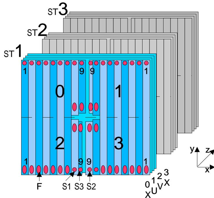
**Figure 1.5:** Schematic layout of the OT: It consists of three stations, each of which contains four layers in an  $xuvx$  configuration. A layer can further be subdivided into left and right halves which are mounted on aluminium frames that can be retracted from the beam pipe for maintenance. Each half consists of nine modules. Separate readouts for the top and the bottom half of each module make it feasible to partition an OT layer into quarters, as shown in the picture.
