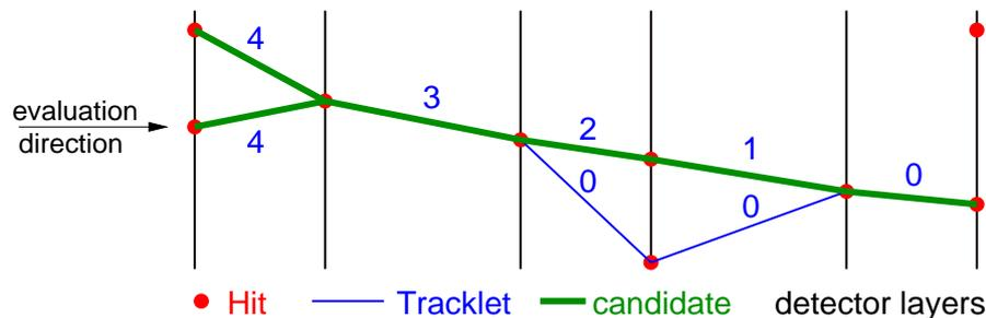
**Figure 4.5:** Sketch of the state of the automaton after candidates have been formed: Two candidates can be seen which only differ in one tracklet (thick green lines).
