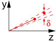
For all pseudo- $x$  clusters, the  $y$  coordinate of the second measurement must be within a window  $\delta$  around the line in  $yz$  projection which joins the first measurement of the pseudo- $x$  cluster with the origin. Effectively, this imposes the restriction that the pseudo- $x$  cluster points to the primary vertex in  $yz$  projection.
