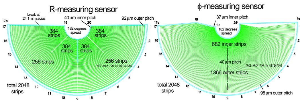
**Figure 1.2:** Schematic view of the two types of Velo sensors. The one shown on the left measures the radial distance of a particle to the beam, the right one measures the azimuthal angle.
