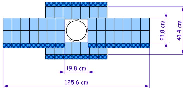
**Figure 1.4:** Sketch of an  $x$  layer in the IT. It consists of several sensors located around the beam pipe.
