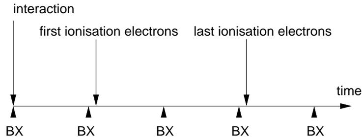
**Figure 1.7:** Sketch illustrating the arrival of drift electrons at the wires in the OT with respect to the time when the primary interaction happened. The corresponding bunch crossing is the first one shown; the small arrows labelled “BX” below the time axis also indicate the following ones.
