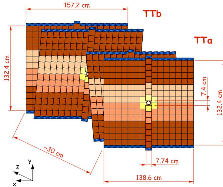
**Figure 1.3:** Layout of the TT stations. The two stereo layers in the middle are called  $u$  and  $v$  layers.
