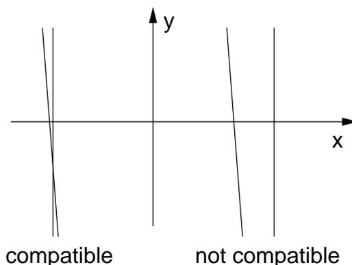
**Figure 2.4:** Straws in  $x$  and stereo layers are compatible if they overlap in  $xy$  projection (left) and incompatible if they do not (right). Since  $x$  and stereo layers are separated by a small distance in  $z$ , the change in  $x$  coordinate of tracks over that distance needs to be taken into account as well.
