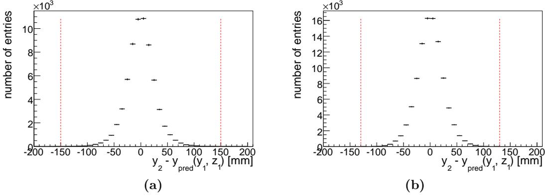
**Figure 5.14:** Plot showing difference of prediction of  $y$  position of second stereo cluster and prediction of that position from first stereo cluster and a vertex assumption. (a) is for “long”, (b) is for “short” best pseudo- $x$  clusters.
