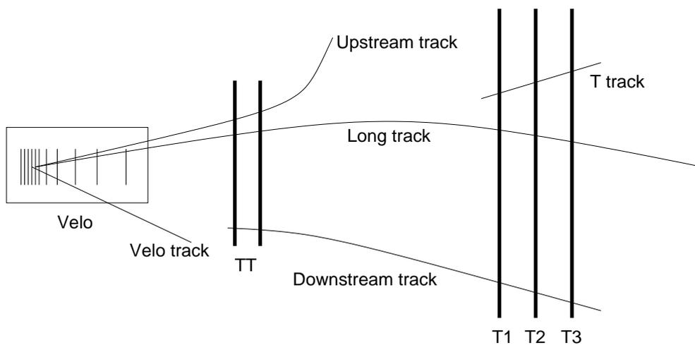
**Figure 2.1:** Schematic view of the track types in the LHCb tracking system.
