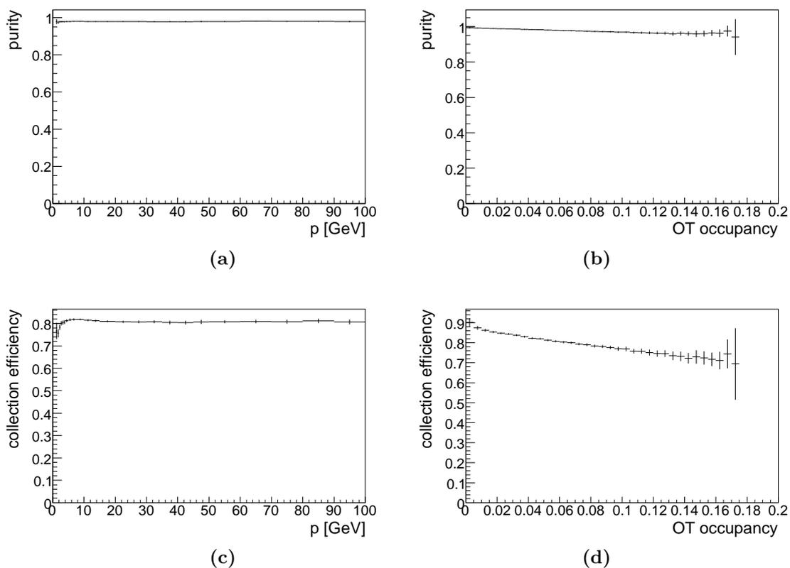
**Figure 6.6:** Purity (top row) and measurement collection efficiency (bottom row) for the standard algorithm on the ALL sample. On the left, the plots versus momentum are shown, those on the right are versus OT occupancy. Purity is stable with respect to momentum and occupancy. The collection efficiency worsens slightly for low momenta and high occupancies, but in a more pronounced way than for the cellular automaton.
