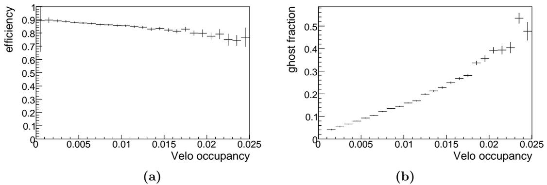
**Figure 3.6:** Reconstruction efficiency (a) and ghost fraction (b) for Long tracks found by the Forward Tracking against Velo occupancy.
