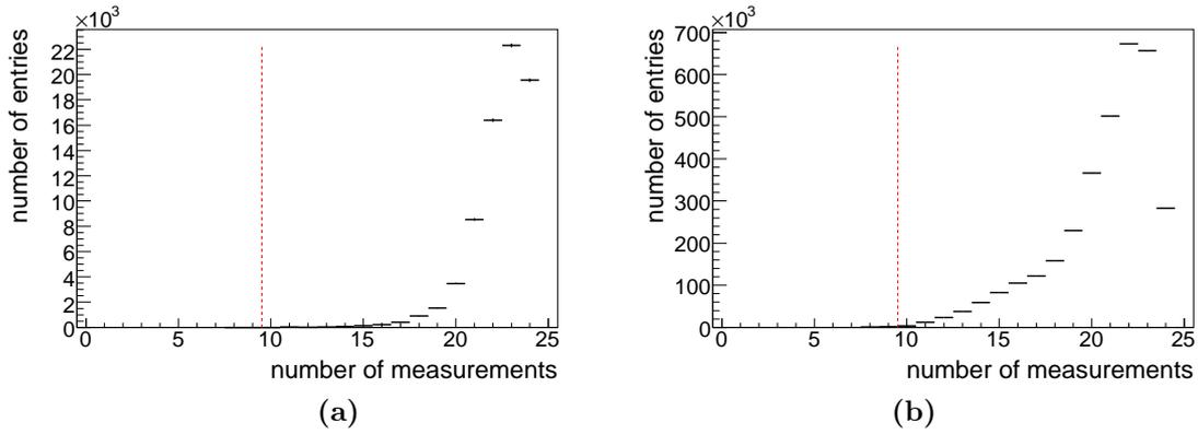
**Figure 5.26:** Number of measurements per candidate. (a) is for best candidates, (b) for wrong ones. While the cut does little for the five tracklet chains considered here, its effects become stronger for shorter chains.
