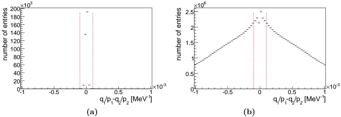
**Figure 5.19:** Distributions of difference in  $q/p$  for two tracklet combinations in adjacent layers. Best combinations (two best tracklets) are in (a), in (b), wrong combinations are shown (at least one bad tracklet or two good tracklets from different particles). One demands that this difference is smaller than  $10^{-4} \text{ MeV}^{-1}$ .
