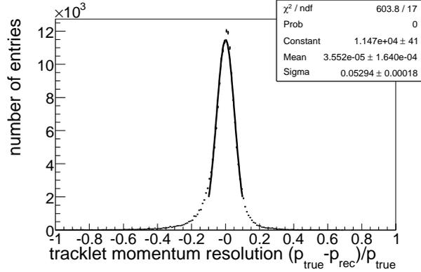
**Figure 5.7:** Momentum resolution  $\Delta p/p$  obtained during the tracklet generation stage using the  $p_T$ -kick method for best tracklets, assuming the tracklet is in the  $y = 0$  plane. The fit to the core of the distribution was done with a single Gaussian.
