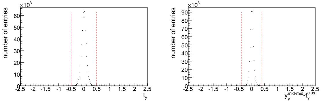
(a) Slope distribution in  $yz$  projection derived from the coordinates of two pseudo- $x$  cluster midpoints for best combinations. (b) Distribution of the difference in slope  $t_y$  between the line joining the two pseudo- $x$  cluster midpoints and the “long” pseudo- $x$  cluster.
