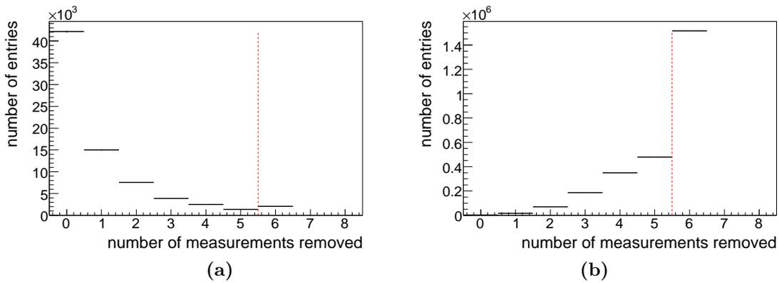
**Figure 5.29:** Number of measurements per candidate removed by the outlier removal. (a) is for best candidates, (b) for wrong ones. The code stops after removing six measurements from a candidate to save time.
