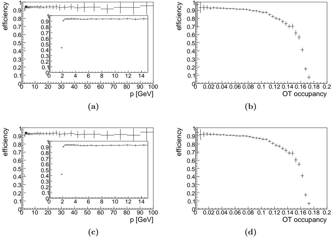
**Figure 6.3:** Event averaged efficiency of the standard algorithm reconstructing only the OT. The top row is for the 6X sample, bottom row for the ALL sample. On the ALL sample, efficiency is a little better for higher momenta than for the cellular automaton based algorithm, however, for momenta below 2 GeV this algorithm performs worse on both samples.
