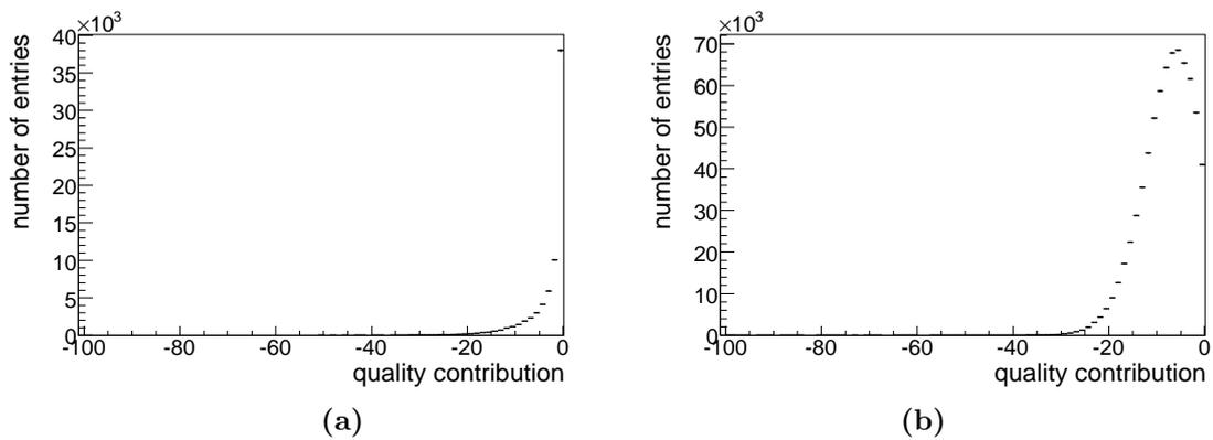
**Figure 5.33:** Contribution from  $\chi^2$ -probability of fit in  $yz$  projection to track candidate quality variable for best reconstructed alternative for particles (a) and ghost candidates (b).
