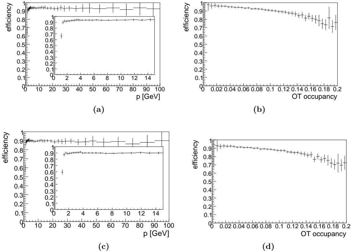
**Figure 6.1:** Event averaged efficiency of the cellular automaton based algorithm, versus momentum (left) and versus Outer Tracker Occupancy (right). Top row is for the 6X sample, bottom row is for the ALL sample. On the 6X sample, the algorithm plateaus around 94 % efficiencies for higher momenta, and performance degrades gracefully for high detector occupancies.
