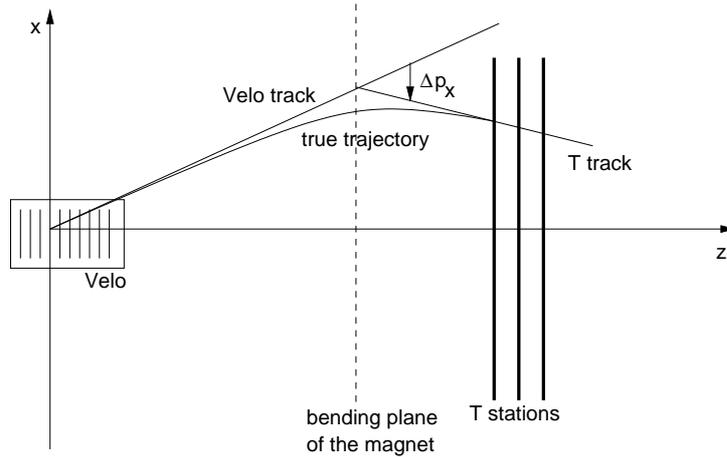
**Figure 2.5:** *It is possible to obtain a momentum estimate from the “kick” that a particle receives in the field of the magnet.*
