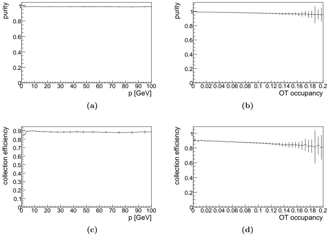
**Figure 6.5:** Purity (top row) and measurement collection efficiency (bottom row) for the cellular automaton based algorithm on the ALL sample. On the left, the plots versus momentum are shown, those on the right are versus OT occupancy. Purity is stable with respect to momentum and occupancy. The collection efficiency worsens slightly for low momenta and high occupancies.
