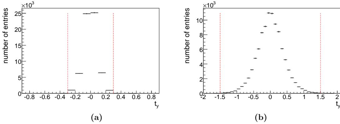
**Figure 5.15:** Slope  $t_y$  for best combinations, calculated using stereo cluster  $y$  positions obtained from stereo coordinate and tracklet in  $xz$  projection. (a) is for “long” pseudo- $x$  clusters. (b) for “short” ones shows the effect of worse spatial resolution in  $y$  and a short lever arm, widening the distribution.
