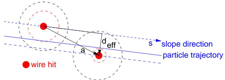
**Figure 5.9:** Calculation of effective pitch.  $\vec{a}$  is the vector joining the two wires,  $\vec{s}$  is a unit vector in direction of the trajectory of the particle. Then, the effective pitch  $\vec{d}_{\text{eff}}$  can be obtained by subtracting from  $\vec{a}$  the projection of  $\vec{a}$  onto  $\vec{s}$ .
