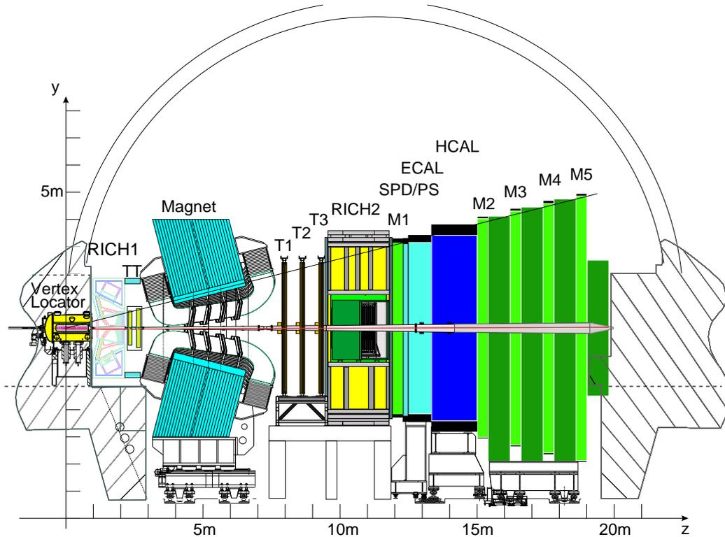
**Figure 1.1:** Side view of the LHCb detector. The positive  $z$  axis points in the direction of the proton beam (to the right in the picture), the  $y$  axis up, and the  $x$  axis points into the drawing plane.
