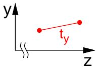
For “long” pseudo- $x$  clusters that were built from stereo layers in different OT stations, the lever arm is long enough to obtain an estimate of the slope  $t_y$  from  $y_u$  and  $y_v$  alone, without assuming anything about the primary vertex.
