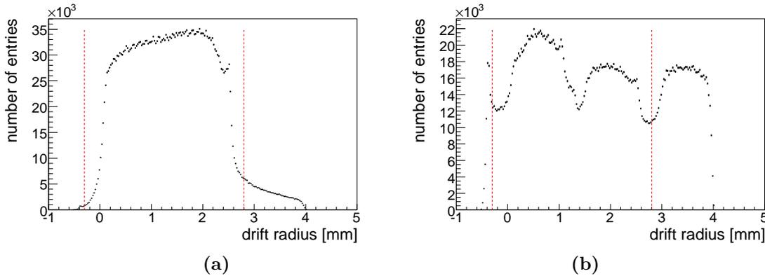
**Figure 5.1:** *Distribution of drift radii as returned by the reconstruction software at this stage of the processing; good measurements are in (a), (b) shows everything else. The structure in the right plot is a consequence of the spillover contribution from other bunch crossings. Dashed red lines will from now on indicate where cuts are performed.*
