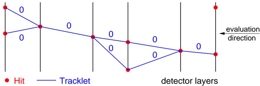
**Figure 4.3:** Sketch of the detector at the end of the tracklet generation phase. Tracklets have been drawn between layers. The state of the tracklets is shown as well. Initially, all tracklets have their counter at zero. The order in which the algorithm processes the individual layers is indicated (“evaluation direction”).
