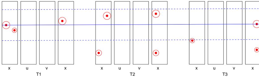
**Figure 2.2:** *Forming search windows. Wires are indicated with a solid red dot, the red circles are the corresponding drift circles. Using two  $x$  measurements, one in  $T1$  and one in  $T3$ , a straight line is constructed. All measurements inside a window around the line (dashed lines) are examined further by the algorithm. (Only measurement in  $x$  layers are shown. Not to scale.)*
