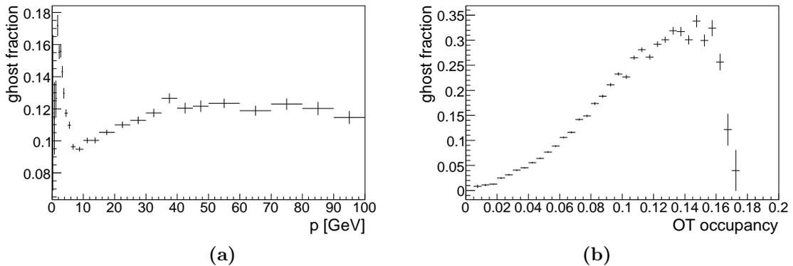
**Figure 6.4:** Event averaged ghost fraction for the standard algorithm. The ghost fraction is shown versus momentum in (a), and versus OT occupancy in (b). The drop at high occupancies is due to the cuts described in 3.2.3.
