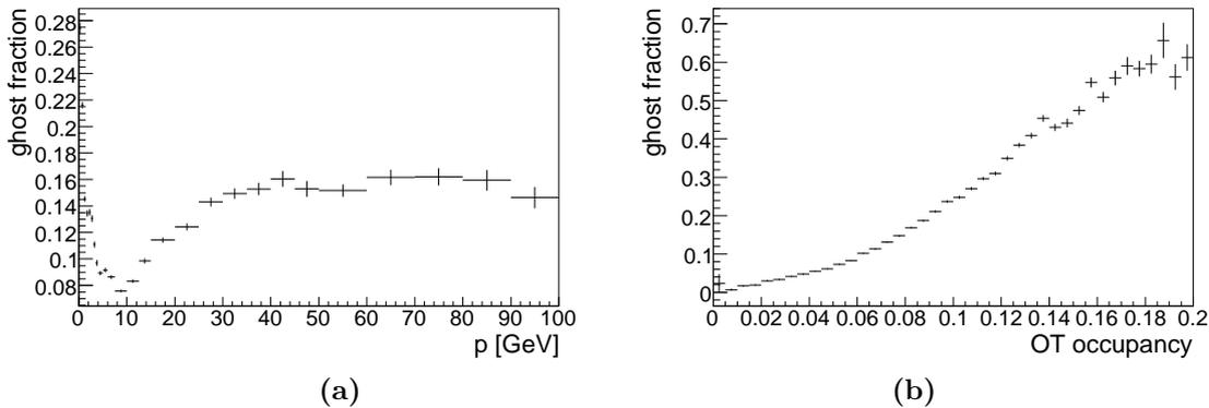
**Figure 6.2:** Event averaged ghost fraction for the cellular automaton based reconstruction algorithm versus momentum (a) and versus Outer Tracker occupancy (b). As can be expected, the ghost fraction rises with occupancy.
