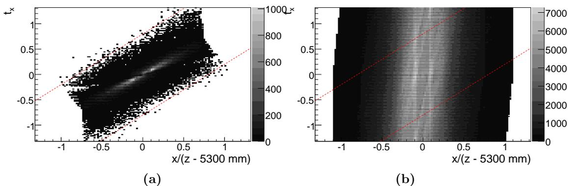
**Figure 5.5:** Scatter plot showing the slope of the line connecting the first measurement of a tracklet with the centre of the magnet versus its slope. Best tracklets are in (a), (b) contains only wrong combinations. One observes that best tracklets only occupy a small portion of the area shown in the plot.
