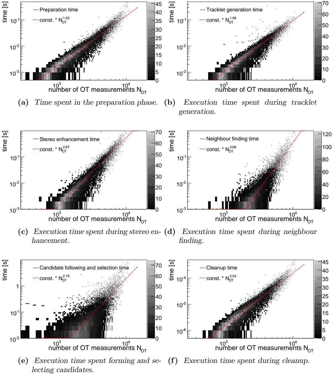
**Figure 6.8:** Execution time spent in the different phases of the algorithm versus number of OT measurements.
