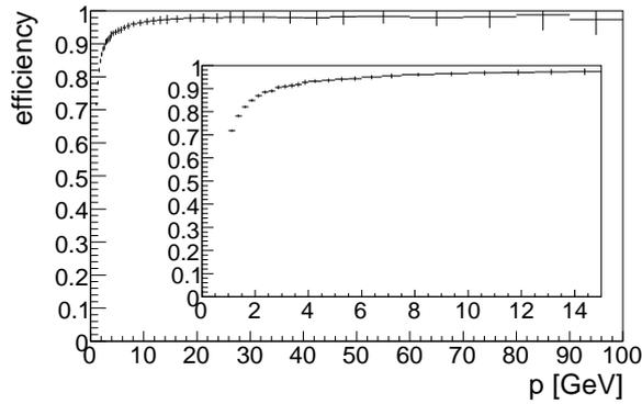
**Figure 3.3:** *Reconstruction efficiency in the Velo against momentum. The inlay plot shows the low momentum end in greater detail. Reconstructed particles with momenta below 1 GeV are not shown in this and subsequent plots.*
