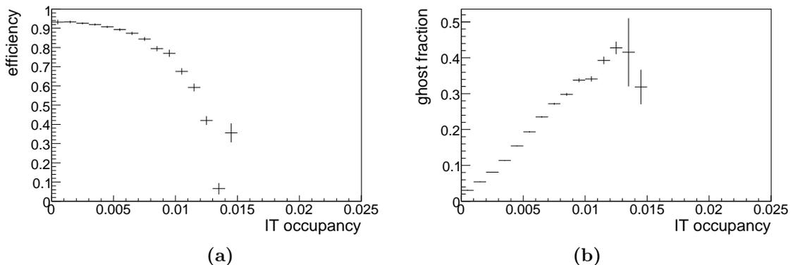
**Figure 3.8:** Reconstruction efficiency (a) and ghost fraction (b) for  $T$  tracks found by the  $T$  station seeding against IT occupancy. Both curves drop at high occupancy (cf. Fig. 3.2a) because of cuts applied in the algorithm (see text).
