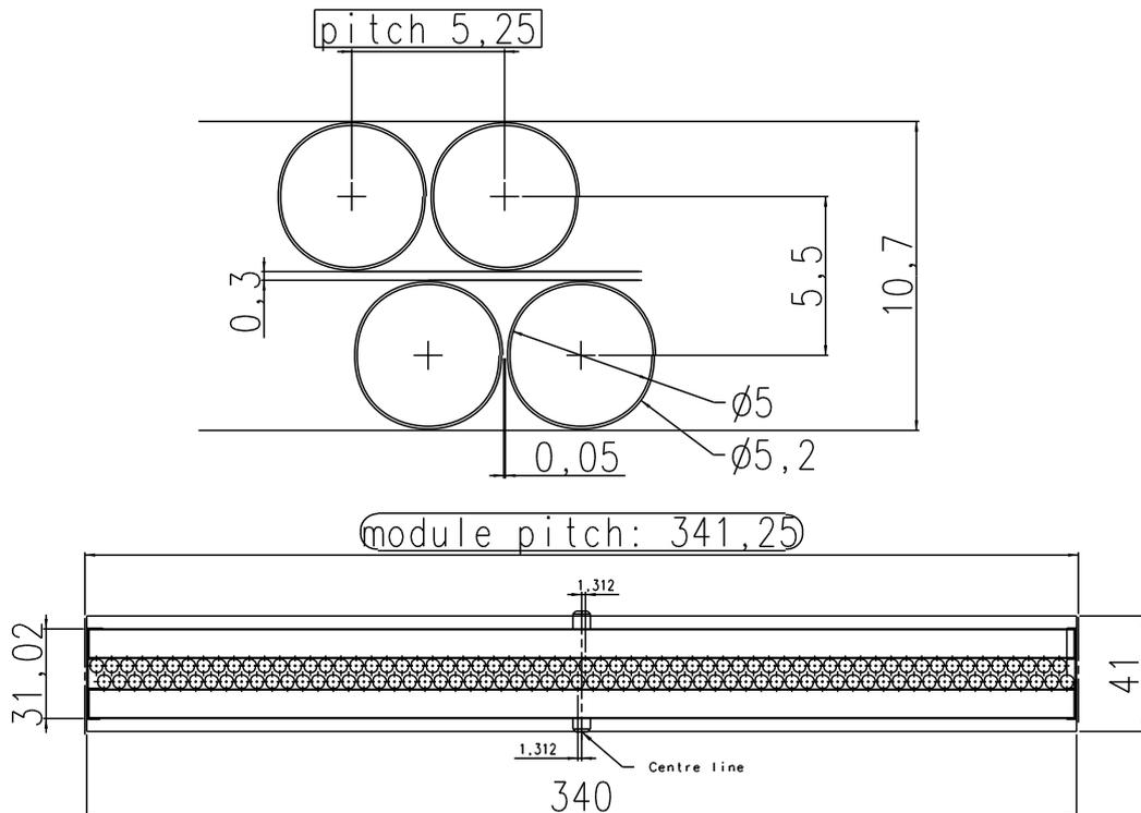
**Figure 1.6:** Cross section through a module used in the Outer Tracker. A module consists of two monolayers of straws which are staggered such that the insensitive areas between the straws in two monolayers do not coincide. The upper part of the drawing shows a magnified part, illustrating how straws are mounted in detail, the lower part gives an impression of the overall module dimensions (all lengths are measured in millimetres). A typical module is about 5 metres long.
