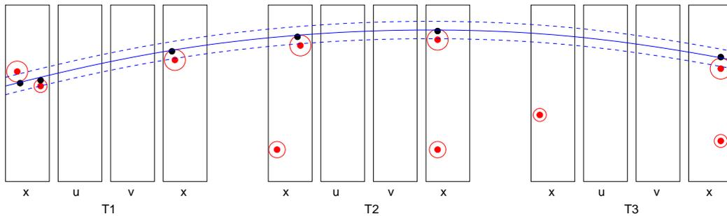
**Figure 2.3:** *Selecting an  $x$  measurement in  $T2$  in addition to those selected in  $T1$  and  $T3$ , eight parabolas are constructed, one for each combination of ambiguities of the three selected measurements. One such parabola is shown, the ambiguities chosen are symbolised by black dots. The measurements inside a tighter window around the parabola (dashed lines) are counted. (Only measurement in  $x$  layers are shown. Not to scale.)*
