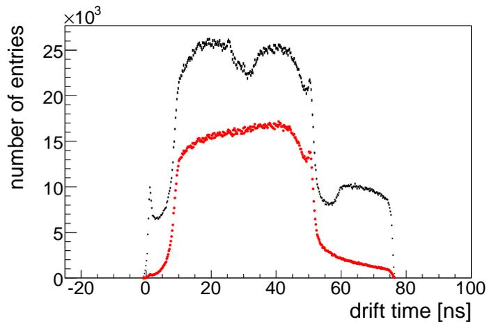
**Figure 1.8:** Drift time spectra in the simulation: The black curve shows all measurements inside a three bunch crossing window, the red one is the part of the spectrum caused by particles from the bunch crossing one is interested in. A time of flight correction has been applied to the data. The tail for long times in the red curve may be due to low momentum particles for which the time of flight correction is biased.
