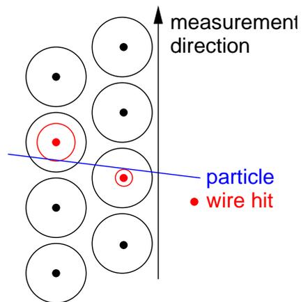
**Figure 5.3:** Sketch of a typical cluster formed by a particle travelling through an OT module (only the straws themselves are drawn). Drift circles have been added for the straws giving a measurement.
