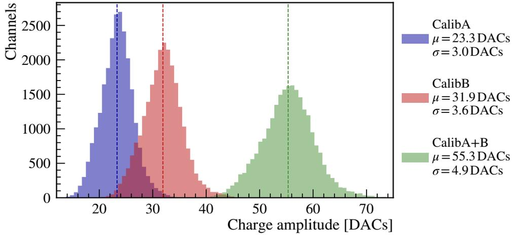
**Figure 6.4:** Amplitude distributions of the three charge values available through the internal charge injection mechanism. The mean values are indicated by the dashed lines.
