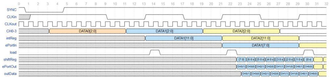
**Figure 4.11:** Digital timing diagram of the PACIFIC serialiser during normal operation. The  $x$ -axis is labelled in units of the 320 MHz clock period (CLKout) that determines the output data stream. Image taken from Ref. [74].
