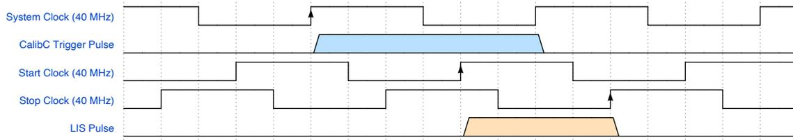
**Figure 4.20:** Timing diagram of the LIS pulse generation in the HK FPGA. The system clock and CalibC pulse are received from the Master GBTX. The start and stop clocks are provided by the third Data GBTX on the Master Board.
