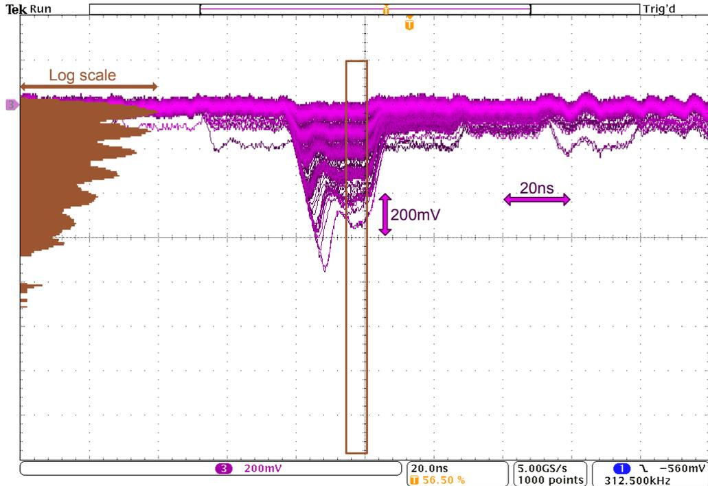
**Figure 4.9:** Typical output of the track and hold stage of the PACIFIC channels. The distribution on the left represents the pulse height projection of the signals within the brown rectangle in logarithmic scale.
