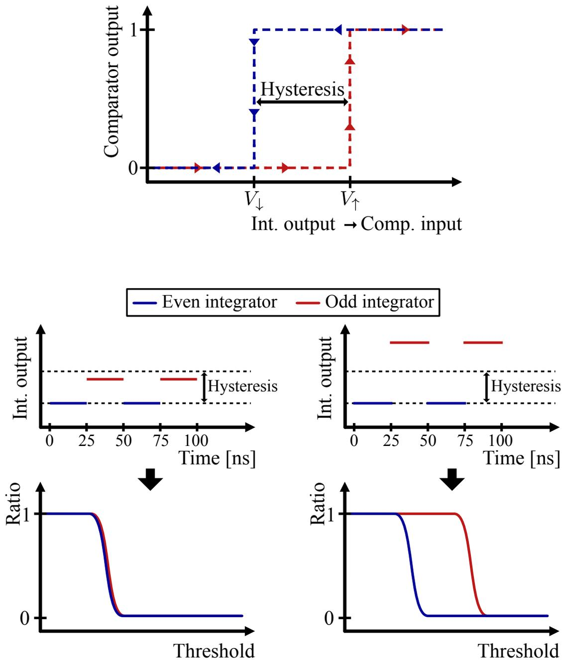
**Figure 6.5:** Illustration of the switching process of the PACIFIC comparator output depending on the input voltage in the presence of a hysteresis (top). Shown below are the consequences that arise from it during a threshold scan for the cases where the even and odd integrator levels are within the hysteresis (left) and exceeding it (right). Note: The output of the integrator (Int.) is fed to the input of the comparator (Comp.).
