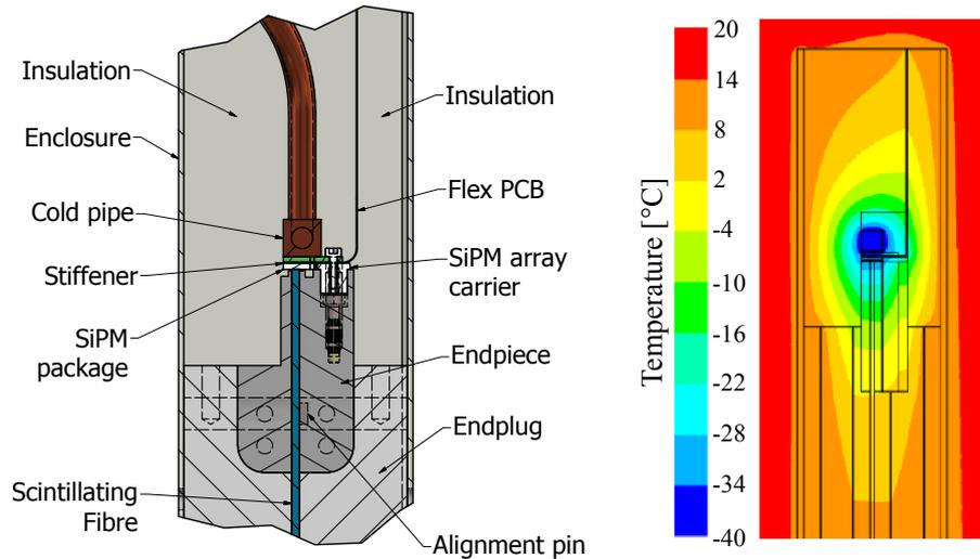
**Figure 3.20:** Cross-sectional view of a SciFi cold box with its components (left), as well as a thermal simulation (right). The SiPM signals are transmitted through the flex PCB to the front-end electronics located above. Images adapted from [20].
