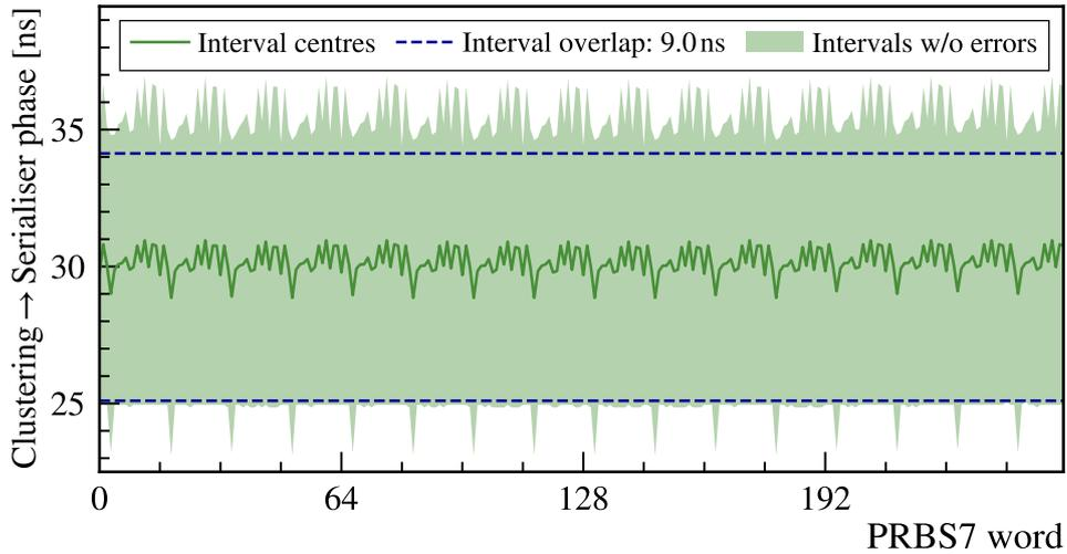
**Figure 5.34:** Error-free intervals in the phase between the Cluster FPGA Clustering and Serialiser blocks for an exemplary ROB. The data within each individual Cluster FPGA and thus clock domain crossing is composed of 16 PRBS7 words.
