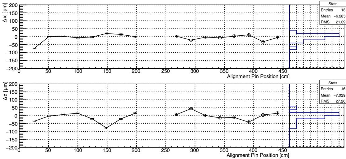
**Figure 3.11:** Evaluation of the straightness of two facing fibre mats within a fibre module using a test setup consisting of a laser and a beam camera. The deviations from a straight line along the alignment pins are shown in both the  $x$  (top) and  $z$  (bottom plot) direction within the LHCb coordinate system.
