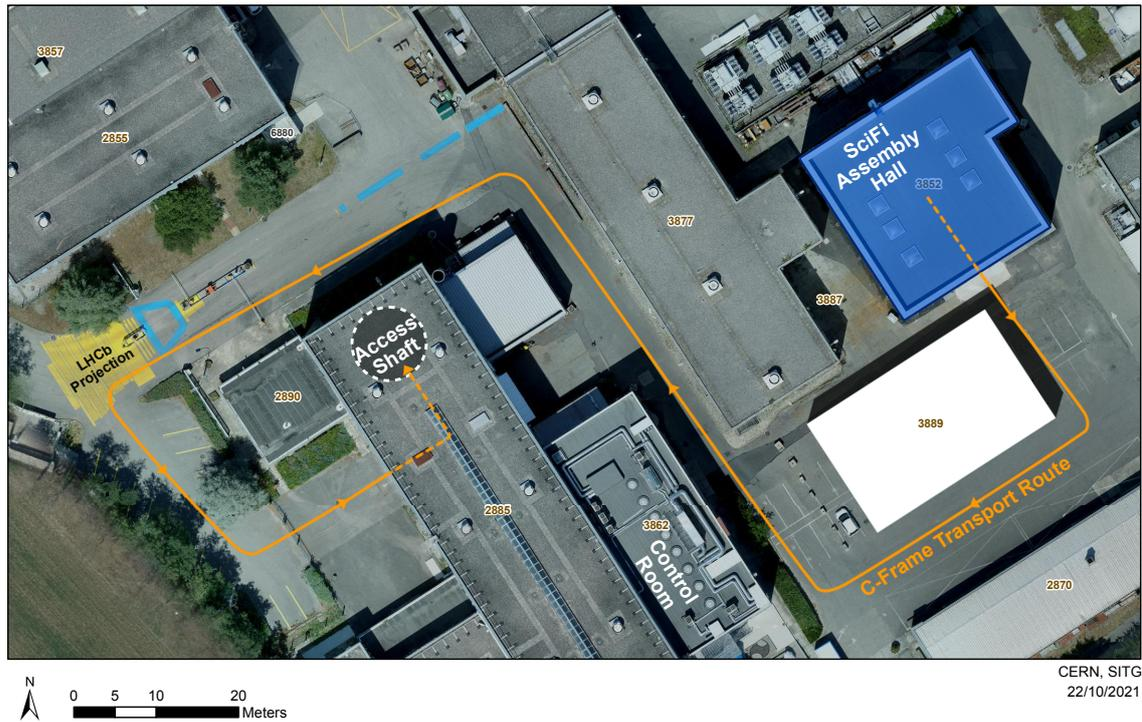
**Figure 5.1:** Location of the SciFi assembly hall, highlighted in blue, at CERN LHC Point 8. The orange path indicates the transport route of the fully assembled and commissioned C-Frames to the access shaft in order to be lowered into the LHCb cavern. The street art on the left shows a projection of the LHCb experiment located 100m underground. Satellite image taken and modified from Ref. [103]
