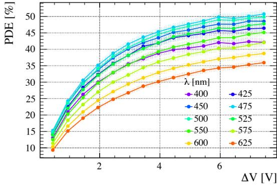
**Figure 3.15:** Measured photon detection efficiencies (PDE) based on a pulse counting approach for an H2017 SiPM array for different wavelengths  $\lambda$  and overvoltages  $\Delta V$ . Image taken from Ref. [57].
