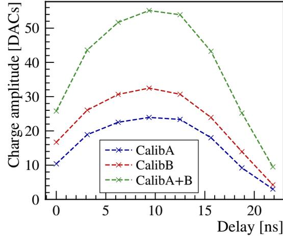
**Figure 6.3:** Internal charge injection amplitudes depending on the delay for an exemplary PACIFIC channel. The amplitudes of the three possible charge values are shown.
