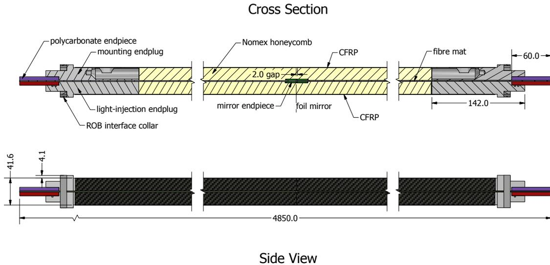
**Figure 3.12:** Cross section and side view of a fibre module of the SciFi Tracker. The dimensions shown in this image are given in mm. Image taken from Ref. [52].
