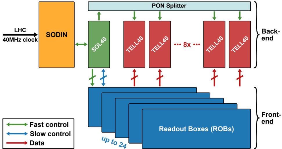
**Figure 5.8:** Interplay of the back- and front-end electronics in the upgraded LHCb DAQ system as used for the commissioning. During the commissioning, the functionality of the SODIN and SOL40 is combined within a single FPGA.
