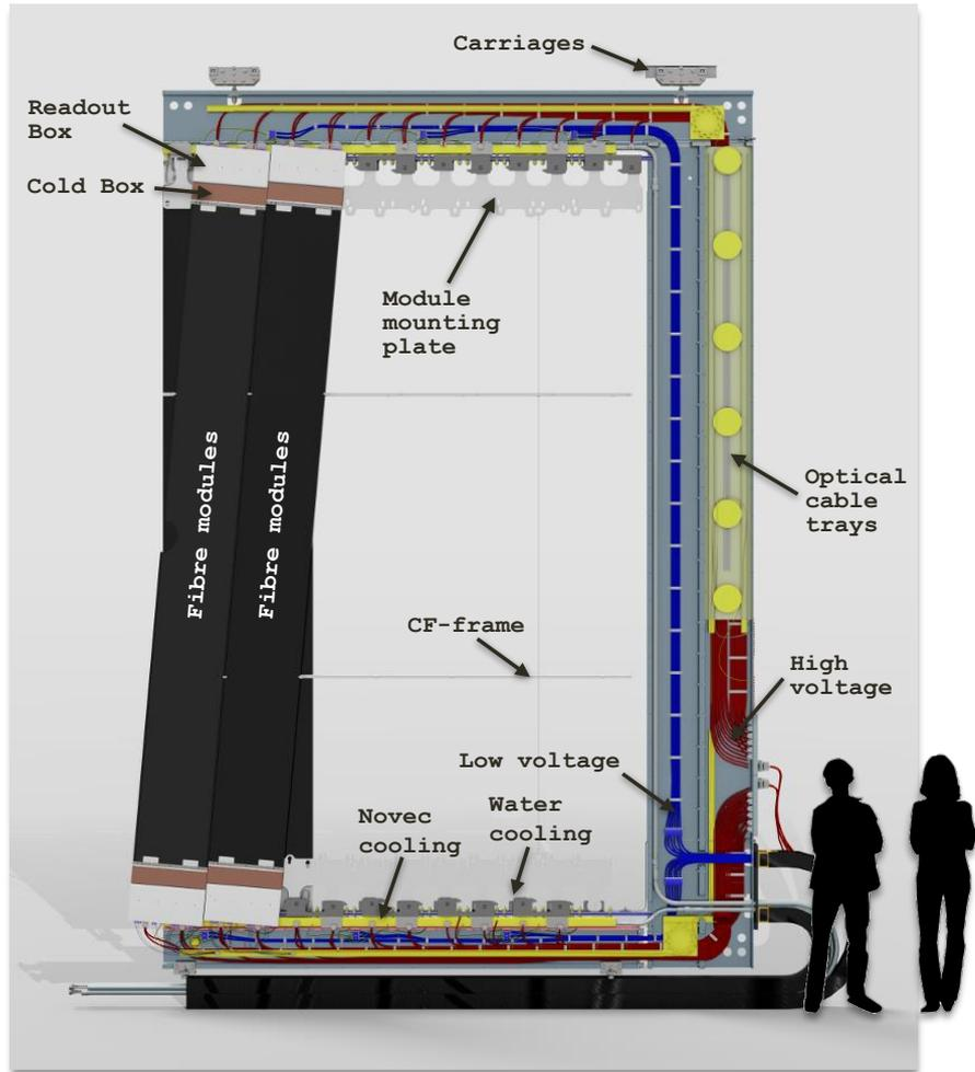
**Figure 3.21:** Schematic illustration of a C-Frame of type SX that carries the detector modules, front-end electronics, and the various infrastructure components. The SciFi Tracker consists of 12 of these frames. Image adapted from Ref. [66].
