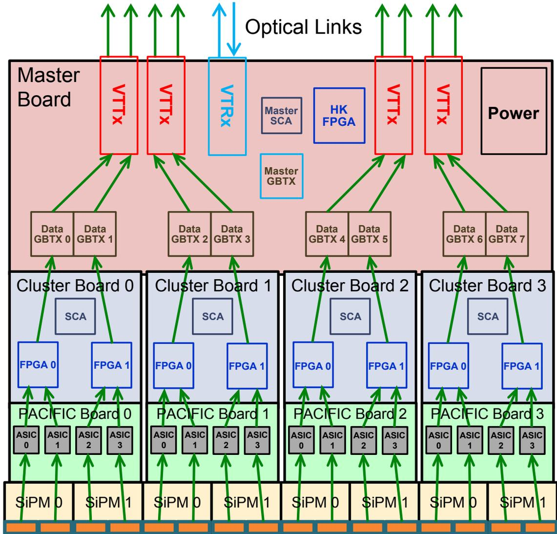
**Figure 4.1:** Block diagram of a HalfROB with the main components on each board denoted. The data stream is indicated by the green arrows. The blue arrows illustrate the bidirectional optical control link. Image edited from Ref. [70].
