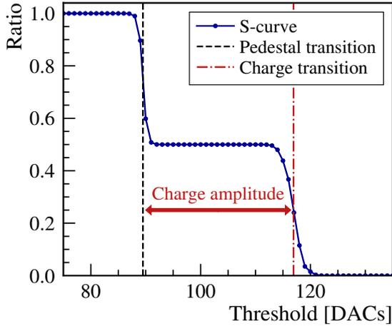
**Figure 6.2:** Typical S-curve when injecting a fixed charge 50% of the time using the internal charge injection mechanism for an exemplary PACIFIC channel.
