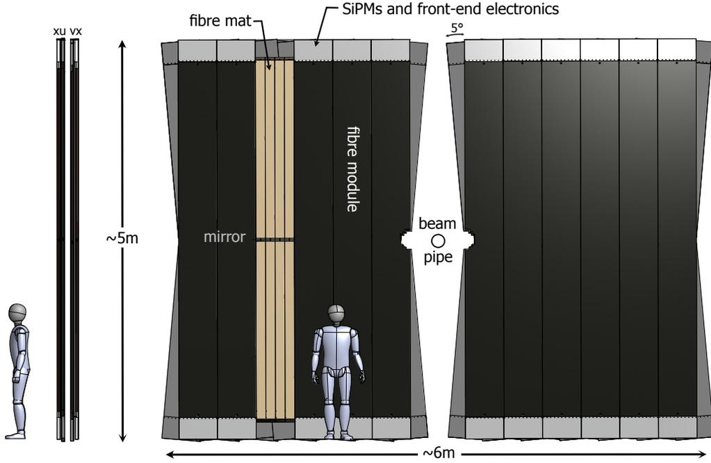
**Figure 3.1:** Schematic side (left) and front (right) view of the SciFi tracking station T3 with a 1.86 m tall human dummy for scale. Image adapted from Ref. [43].
