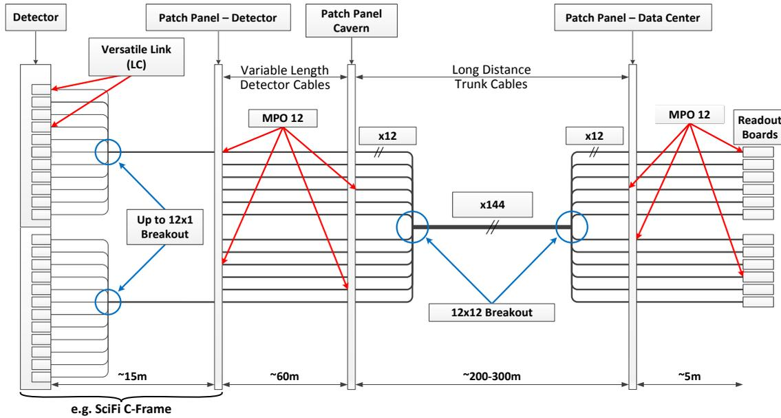
**Figure 5.17:** Fibre system layout for the readout and control of the front-end electronics of the upgraded LHCb experiment. The complete system will contain about 15 000 individual active fibres [34]. With 4096 data and  $2 \times 512$  control fibres, the SciFi Tracker contributes more than 30 % to that. Image adapted from Ref. [112].
