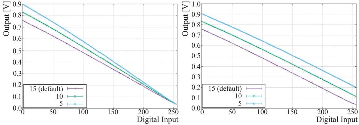
**Figure 4.10:** Relationship between the digital input value and the output voltage of a PACIFIC threshold DAC. In addition, the effect of the slope (left) and offset (right) control is illustrated. Images adapted from Ref. [74].
