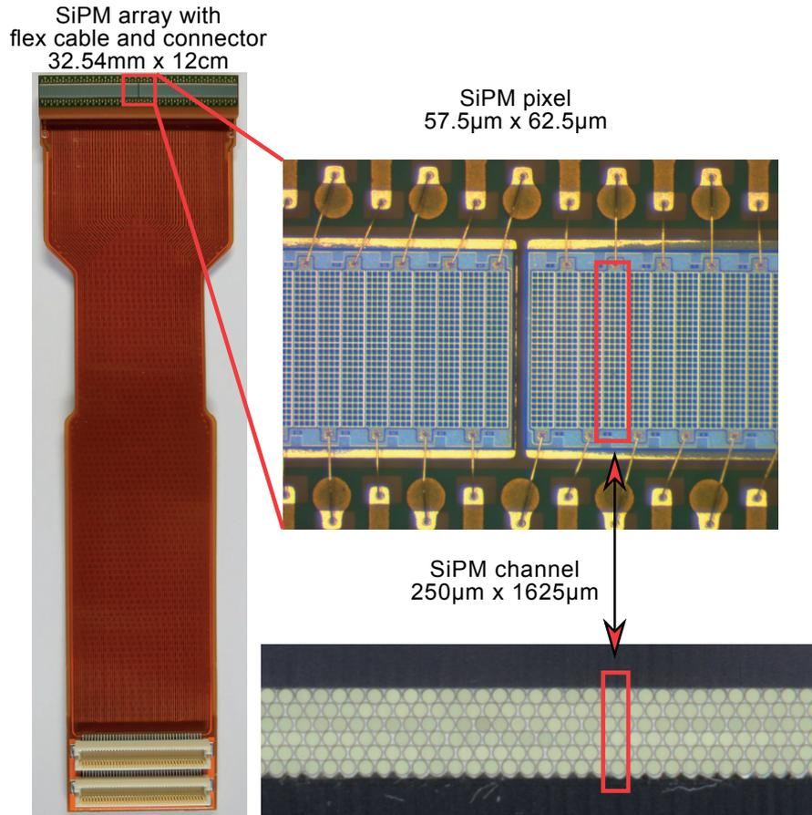
**Figure 3.14:** Hamamatsu H2017 128-channel SiPM array with flex cable and connector as used for the SciFi Tracker (left). A zoomed in view on the active area with the gap between the two dies is shown on the right, as well as an illustration of the position of one SiPM channel with respect to the fibre mat. Image adapted from Ref. [59].
