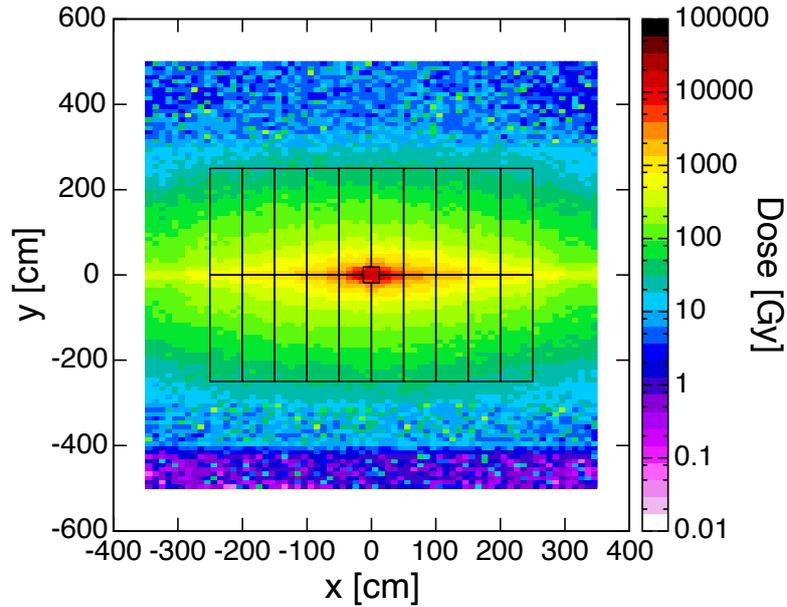
**Figure 2.5:** Expected dose in the  $x$ - $y$  plane at  $z = 783$  cm after an integrated luminosity of  $50 \text{ fb}^{-1}$ . The Scintillating Fibre (SciFi) modules of the first tracking station located at this position are shown superimposed. The integrated dose absorbed in the fibres towards the centre peaks at about 35 kGy. Image modified from [20].
