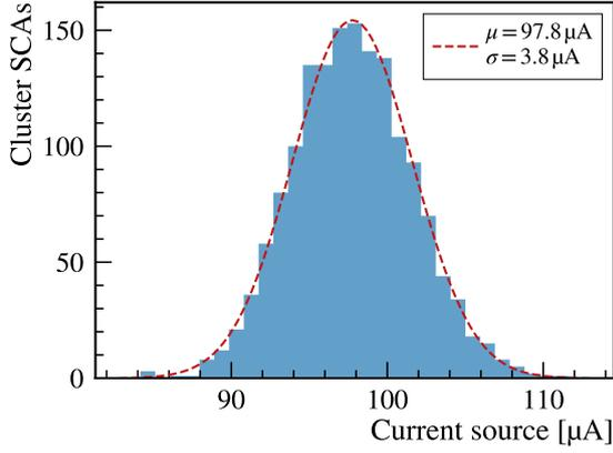
**Figure 5.19:** Distribution of the currents as generated by the Cluster SCAs of the 196 ROBs installed on C-Frames 1 to 9. Measured as part of the FE-Tester test procedure. A Gaussian fit is overlaid.
