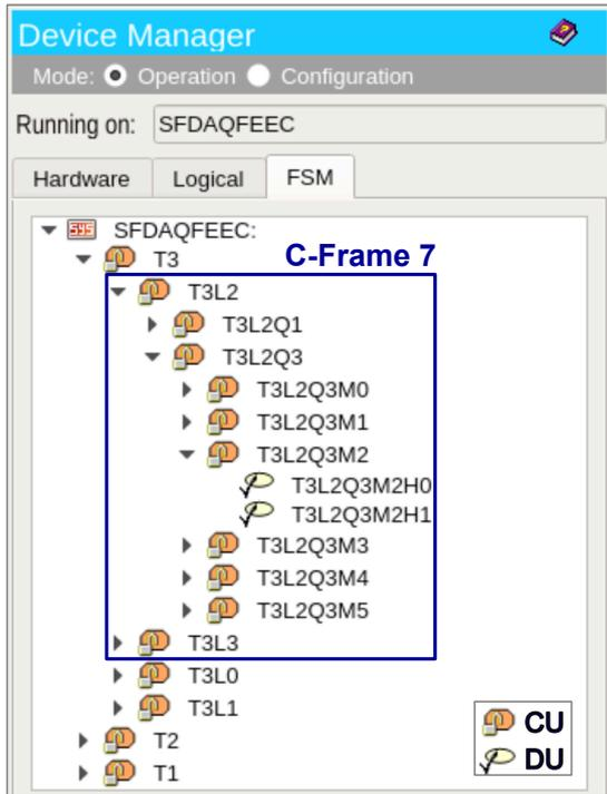
**Figure 5.11:** Screenshot of the device manager used to create and control the hierarchical structure of the SciFi front-end electronics.
