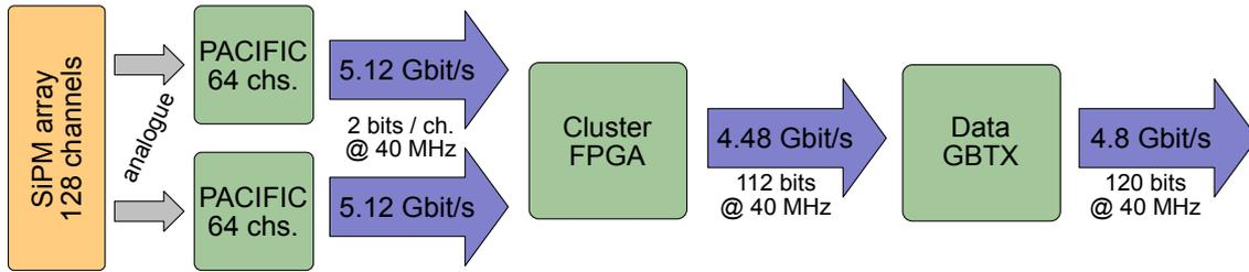
**Figure 4.18:** Data stream and corresponding bandwidths between the different components of the SciFi front-end electronics. In total, 4096 instances of the shown chain are present in the detector, resulting in a total data rate of about 20 Tbit/s arriving at the back-end.
