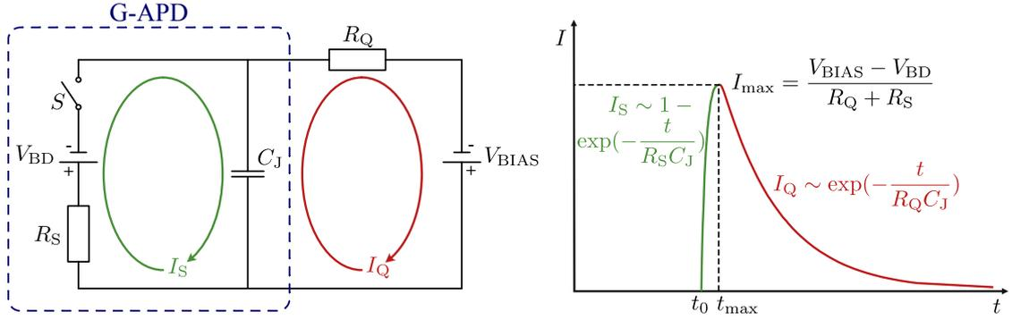
**Figure 3.13:** Electrical circuit of a basic equivalent model for an externally biased G-APD (left). The plot on the right shows the signal pulse after closing (at  $t_0$ ) and re-opening (at  $t_{\max}$ ) the switch  $S$ . Image inspired from Ref. [58].
