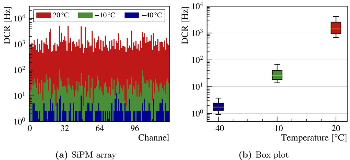
**Figure 6.10:** Dark count rate (DCR) along the 128 channels of one SiPM array for different SiPM temperatures (a). The box plot (b) shows the measured rates for the 192 SiPMs located on the bottom half of C-Frame 2. The box boundaries indicate the 25th and 75th percentiles, in addition to the median (50th percentile) as the orange lines inside the boxes. The whiskers mark the 5th and 95th percentiles.
