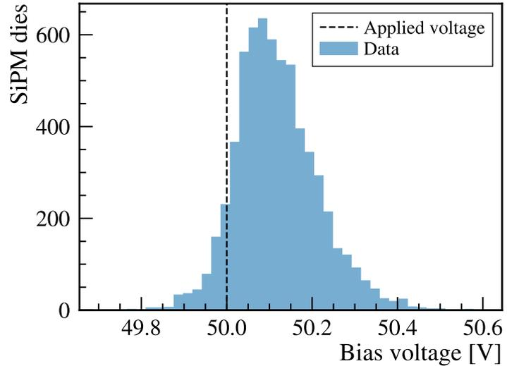
**Figure 5.25:** Monitored bias voltages applied to the SiPM dies of C-Frames 1 to 9.
