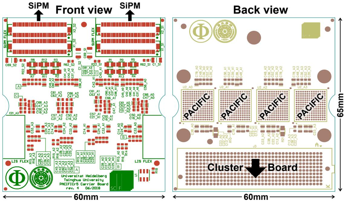
**Figure 4.2:** Layout of the front (left) and back (right) of a PACIFIC Board. The connectors to the SiPM flex cables are shown on the top left. On the bottom right, the FMC connection points to the Cluster Board are displayed. The four PACIFIC ASICs are soldered on the square areas on the right. Image edited from Ref. [71].
