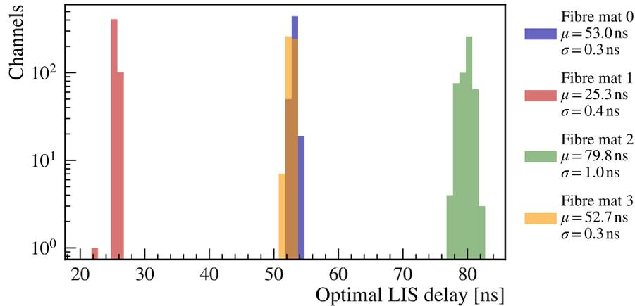
**Figure 5.41:** Distribution of the optimal LIS delay for an exemplary ROB based on the ratio of events above the lowest threshold corresponding to about 1.5 pe.
