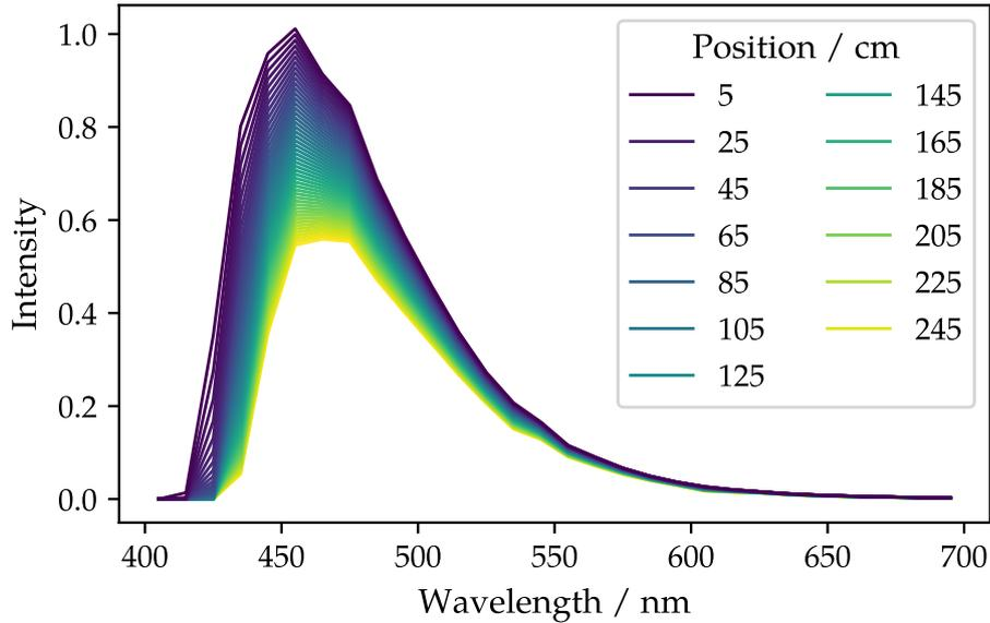
**Figure 3.4:** Emission spectrum of a scintillating fibre of type SCSF-78MJ at different distances to the point of excitation. For short distances, the maximum is located at around 450 nm and shifts towards larger wavelengths with increasing distance due to self-absorption of the inserted wavelength shifter. Image taken from Ref. [50].
