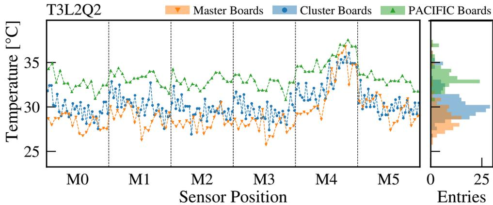
**Figure 5.21:** Temperature readings of the front-end electronics located on T3L2Q2. With the help of this plot as presented in the automated commissioning report, a mounting deficiency of the ROB T3L2Q2M4 was identified.
