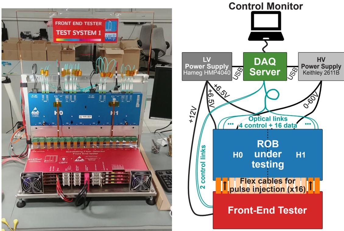
**Figure 5.4:** Photograph of the SciFi Front-End Tester with a mounted ROB under testing (left). A schematic drawing of the complete setup including the DAQ system and power supplies is shown on the right. Two of these test systems are used to verify the proper functioning of the ROBs before being installed on the C-Frames.
