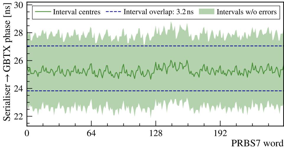
**Figure 5.32:** For an exemplary ROB, the error-free intervals in the phase between the Cluster FPGA Serialiser and the Data GBTX are shown. One ROB comprises 16 individual data links (i.e. 16 different clock domain crossings) with 16 PRBS7 words each, resulting in the total of 256 words and corresponding error counters.
