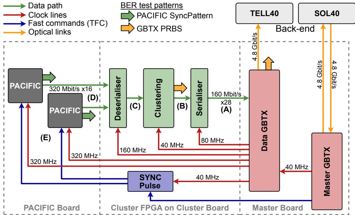
**Figure 5.28:** Clocking scheme of the SciFi front-end electronics. The error-free data transmission relies on the clock domain crossings labelled as (A)–(E). BER test patterns can be generated at three different points along the data path as indicated by the thick arrows.
