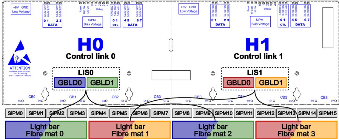
**Figure 5.38:** SciFi ROB cover with the routing of the LIS GBLDs to the fibre mats indicated. Image modified from Ref. [117].
