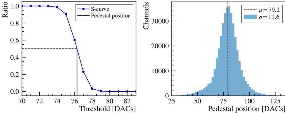
**Figure 5.40:** Exemplary S-curve of one channel without the injection of any signal showing the pedestal transition (left). The position of the pedestal is given by the point on the linear interpolated curve that matches the ratio of 0.5. The distribution on the right shows the determined pedestal positions of the 400k channels within C-Frames 1 to 9.
