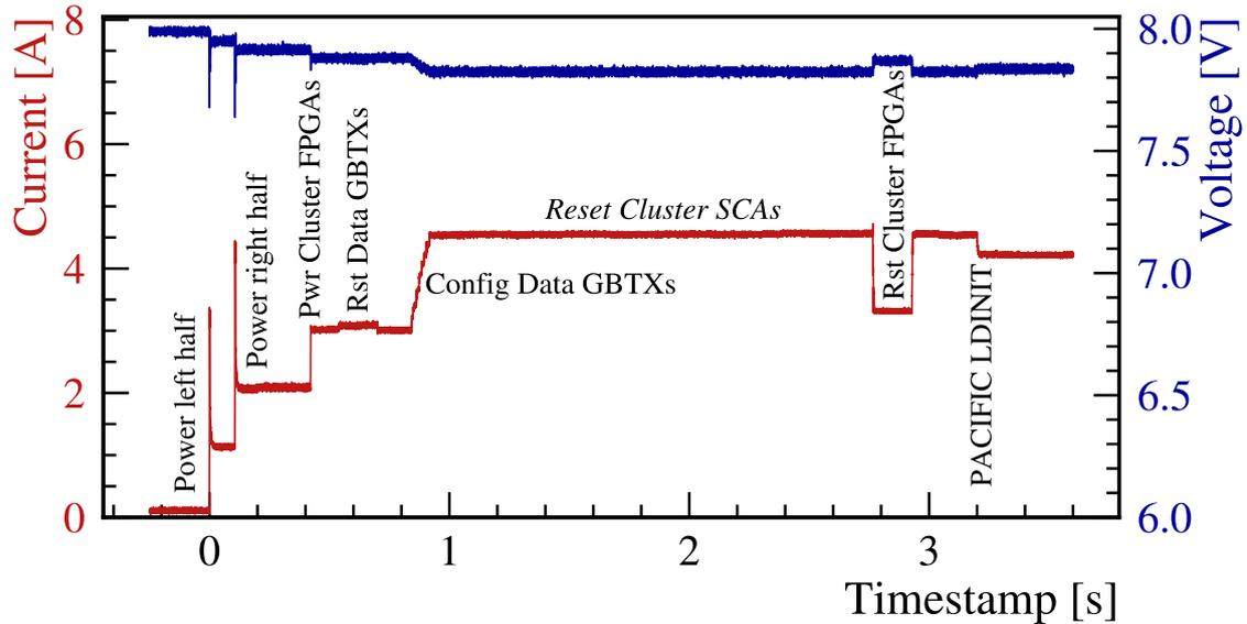
**Figure 5.15:** Time course of the input voltage and current consumption of one HalfROB during the processing of the Reset command as measured with an oscilloscope. The slight changes in the input voltage are due to voltage drops in the power cable itself.
