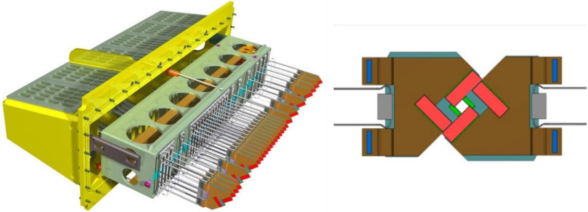
**Figure 2.3:** Schematic view of one half of the upgraded LHCb Vertex Locator (VELO) consisting of 26 modules (left). Two opposing modules from both halves in the closed position are shown on the right. Image adapted from Ref. [26].
