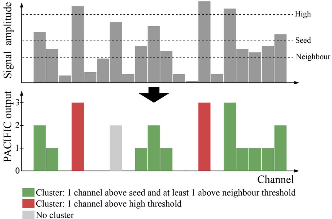
**Figure 4.14:** Illustration of the clustering algorithm. The height of each rectangle at the top depicts the SiPM signal amplitude in one channel. The 2-bit patterns below represent the outputs of the PACIFIC channels after applying the three comparator thresholds. Five clusters are identified by the algorithm as indicated by the green and red colors depending on the fulfilled condition.
