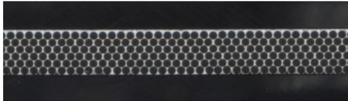
**Figure 3.6:** Cross section of one fibre mat used in the SciFi Tracker. Image taken from Ref. [50].
