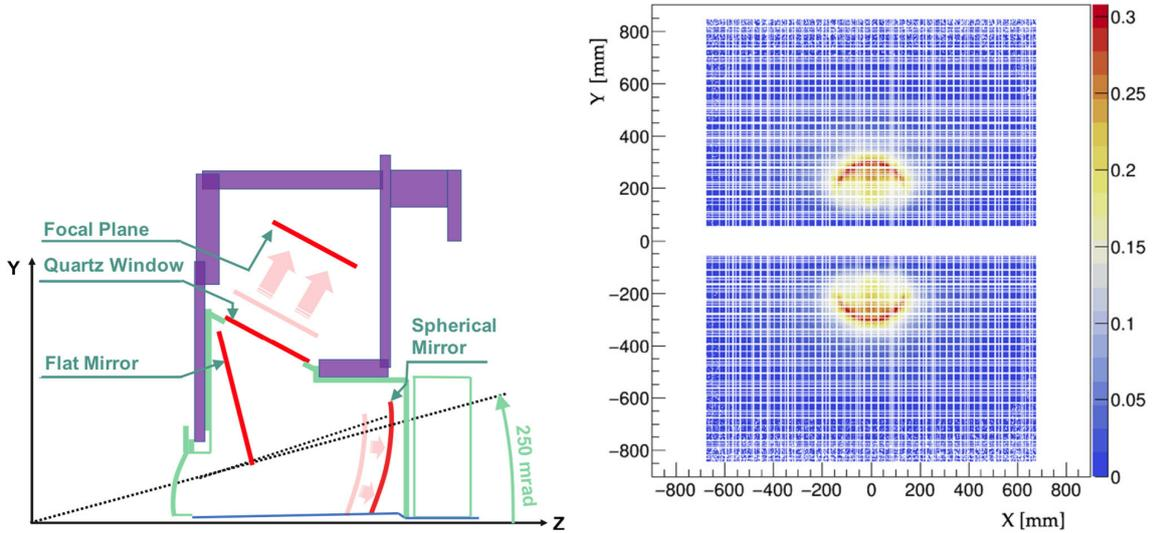
**Figure 2.6:** Schematic side view of the upper half of RICH1 (left) and simulated single channel occupancy (right). Modifications to the mechanical and optical system in the course of the upgrade are indicated by the red arrows in the side view. Images taken from Ref. [29].
