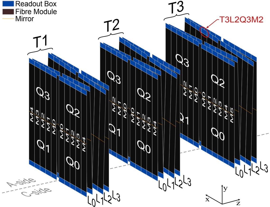
**Figure 5.6:** Schematic view of the SciFi Tracker with the naming convention overlaid. An example ROB and its location identifier is highlighted in red. Distances between the layers (L) and stations (T) are exaggerated for better visibility. The inner layers per station (L1 & L2) are tilted by  $\pm 5^\circ$  to obtain the  $y$ -coordinate of detected hits.
