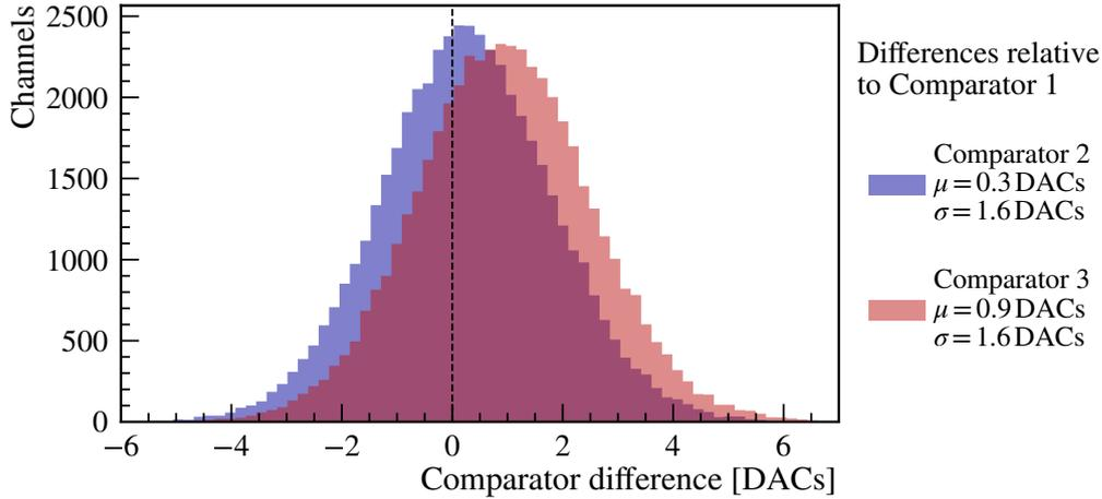
**Figure 6.8:** Differences in the determined charge transitions between the different PACIFIC comparators. The underlying data is taken from the 50k channels on C-Frame 2 using the internal charge injection mechanism. The differences to the (reference) comparator 1 in each channel are displayed. The mean values  $\mu$  and standard deviations  $\sigma$  of the distributions are indicated on the right.
