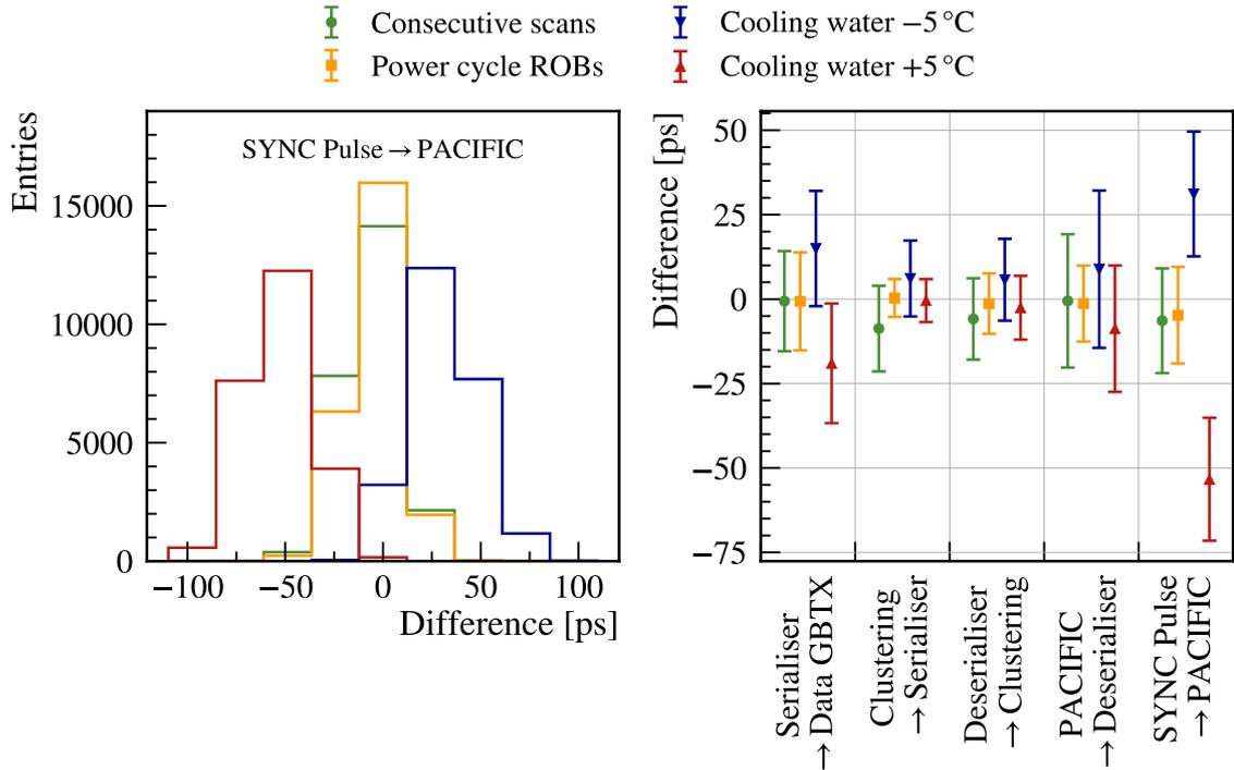
**Figure 6.9:** Differences in the optimal clock phases between the SYNC Pulse and PACIFIC clock for different run conditions compared to a reference (left). Measured by the centres of the error-free intervals. The right plot summarises the mean and standard deviation of the underlying distributions for the remaining clock phases within the SciFi front-end electronics as indicated by the markers and error bars, respectively.
