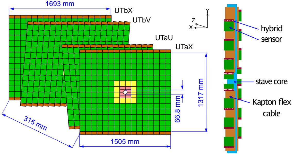
**Figure 2.4:** Schematic layout of the Upstream Tracker (UT) with the four detection layers (left). The detector is composed of four different sensor types: Type A (green), B (yellow), C and D (pink). It is built from vertical staves, which carry the sensors and readout hybrids as shown on the right. Image adapted from Ref. [27].
