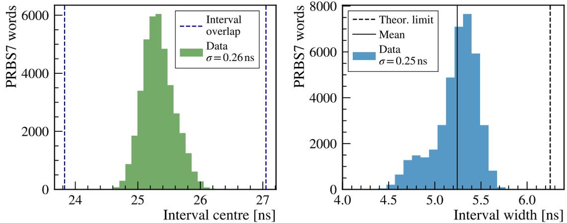
**Figure 5.33:** Error-free intervals in the phase between the Cluster FPGA Serialiser and Data GBTX clock. The distributions of the interval centres (left) and widths (right) include data from 152 ROBs as obtained during the front-end electronics commissioning. The theoretical limit of 6.25 ns on the width results from the transmission speed of 160 Mbit/s per lane.
