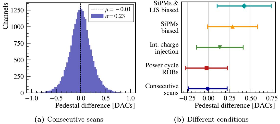
**Figure 6.1:** Variations of the determined pedestal positions between two consecutive threshold scans (a) and under further conditions (b) for the 25k channels of one C-Frame half. The reference scan has been performed with the HV and LIS turned off. In the right figure (b), the mean values  $\mu$  and standard deviations  $\sigma$  of the underlying distributions are indicated by the markers and error bars, respectively.
