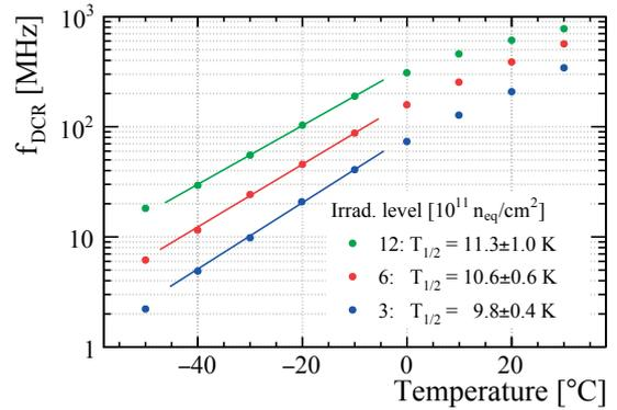
**Figure 3.18:** Dark count rate (DCR) as a function of the temperature for irradiated H2017 SiPMs at  $\Delta V = 3.5$  V. The coefficient  $T_{1/2}$  that describes the temperature difference at which the DCR is reduced by 1/2 is determined with an exponential fit in the range  $[-40, -10]$  °C and indicated by the solid lines. Image adapted from Ref. [61].
