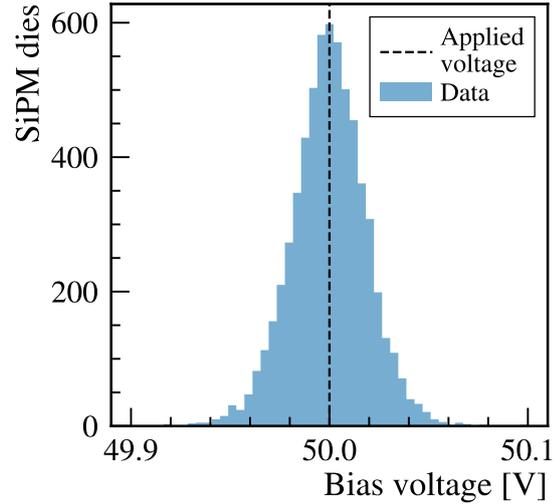
**Figure 5.26:** Linear fit to calibrate the bias voltage monitoring with the determined slope ( $p_1$ ) and intercept ( $p_0$ ) overlaid. **Figure 5.27:** Monitored bias voltages applied to the SiPMs after the HV calibration of C-Frames 1 to 9.
