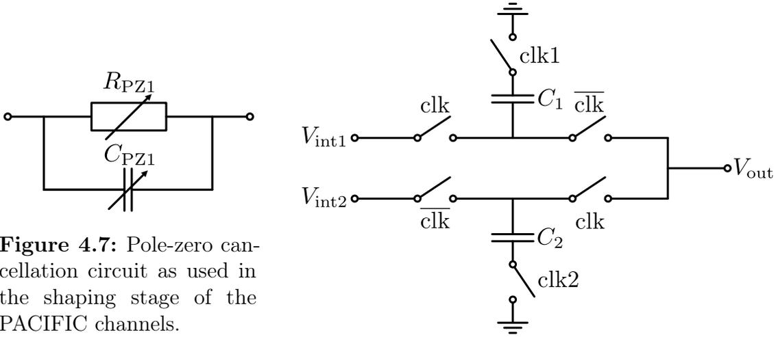
**Figure 4.7:** Pole-zero cancellation circuit as used in the shaping stage of the PACIFIC channels.
