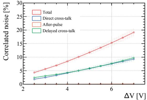
**Figure 3.16:** Probabilities for different types of correlated noise as determined during the quality assurance of 5000 H2017 SiPMs. Variations in the order of  $\pm 1\%$  were observed between the different devices. Image taken from Ref. [61].
