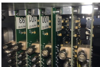
(d) DAQ boards integrated in the bottom part of the telescope.
